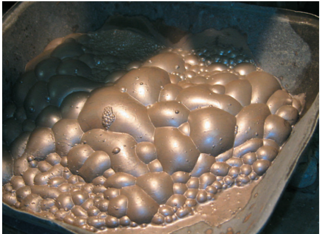
Zn-concentrate flotation test of high grade zinc ore from the Citronen deposit (Ironbark Zinc Limited).
