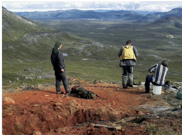
The 'Swan' area of the Qussuk prospect. Channel sampling in the distinct 30 m to 80 m wide band of leached meta-volcanics. Analyses of surface channel samples returned up to 6.5 g/t gold in a 2 m profile, and as much as 0.5 % copper. Courtesy: NunaMinerals.
