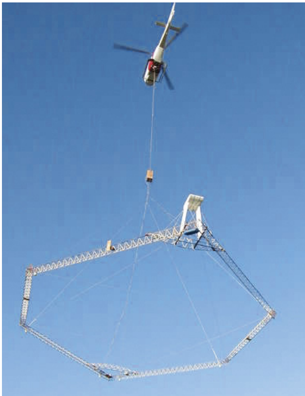
Demonstration by the SkyTEM deep-penetrating helicopter-borne geophysical combined magnetic and time domain transient electromagnetic (TDEM) equipment. Courtesy: SkyTEM.
