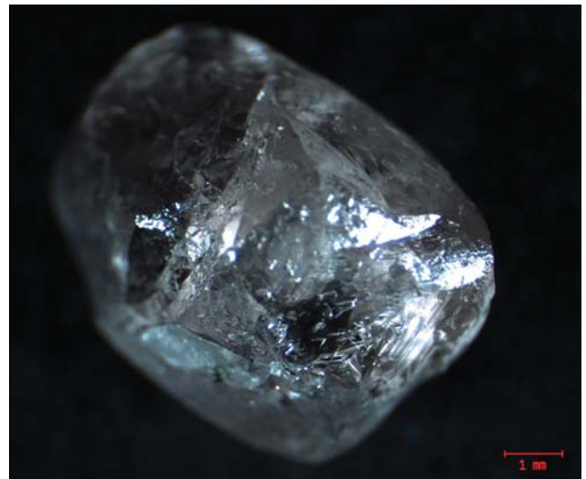
The 2.4 ct stone is described as an off-white, translucent dodecahedral twinned diamond containing inclusions.
