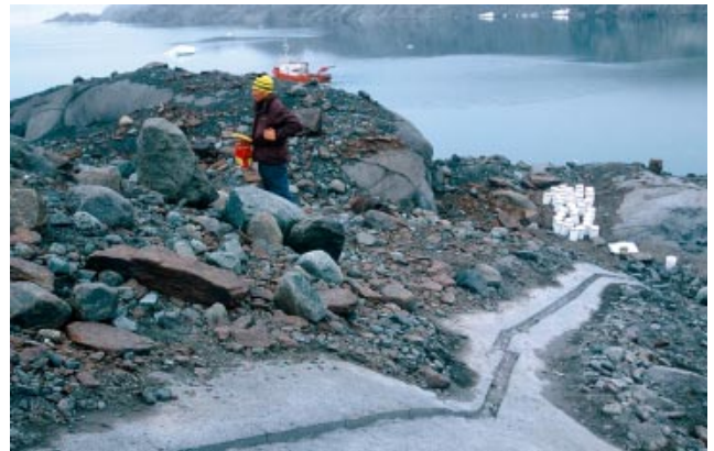
Fig 4: Channel sampling of mineralised layers within the Skaergaard intrusion
