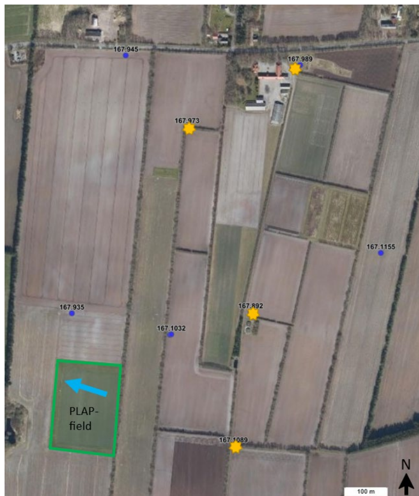
Figure 5.4.4. The location of the PLAP field, Jyndevad delineated by the green box. The yellow stars represent the irrigation wells, and the blue arrow shows the general groundwater flow direction.
