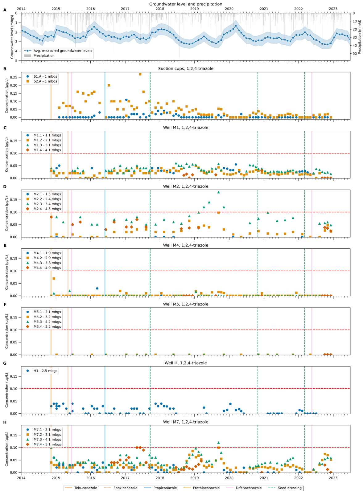
Figure 5.2.1. 1,2,4-triazole monitoring at Jynde vad. Precipitation and measured groundwater levels, with standard deviations (A); measured 1,2,4-triazole in the variably saturated zone (B); measured 1,2,4-triazole in the downstream vertical groundwater monitoring well (C-F); measured 1,2,4-triazole in the horizontal groundwater wells (G); measured 1,2,4-triazole in the upstream vertical groundwater monitoring well M7 (H); The vertical coloured lines indicate the date of azole applications. Azoles applied as seed dressing (vertical green dashed lines). The horizontal red dashed line depicts the limit value of 0.1 µg/L. Note that the results cover the full monitoring period from November 2014 to December 2022. Monitoring of 1,2,4-triazole ended December 2022.
