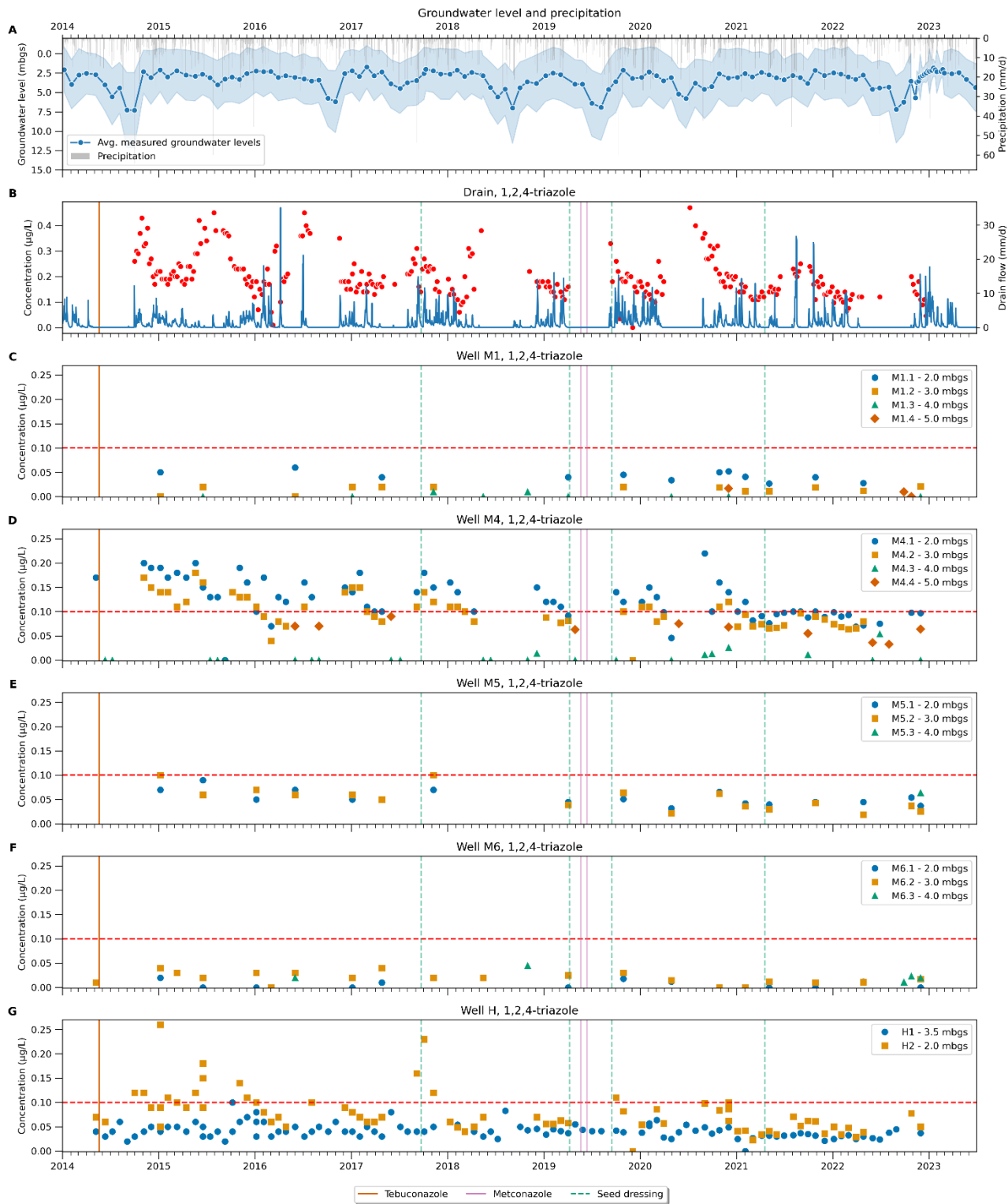
Figure 5.2.3. 1,2,4-triazole monitoring at Estrup. Precipitation and measured groundwater levels, with standard deviations (A); measured 1,2,4-triazole in the variably saturated zone (B); measured 1,2,4-triazole in the downstream vertical groundwater monitoring wells (C-F); measured 1,2,4-triazole in the horizontal groundwater wells (G); It is noted, that sampling of an upstream well at Estrup did not take place during the monitoring period. The secondary y-axis (plot B) represents the drain flow. The vertical coloured lines indicate the date of azole applications. Azoles applied as seed dressing (vertical green dashed lines). The horizontal red dashed line depicts the limit value of 0.1 µg/L. Note that the results cover May 2014-December 2022. Monitoring of 1,2,4-triazole ended in December 2022.
