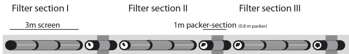
**Figure A8.1.** Design of horizontal well with three filter sections of 3 m (inner diameter 25 mm; outer diameter 32 mm) each separated by 1m packer-section attached 0.8 m bentonite (thickness at installation 1 cm; expand to a thickness of 3.5 cm). Water can be sampled through two PE-tubes (inner diameter 4 mm; outer diameter 6 mm) ending 1 and 2 meters into each section, respectively.
