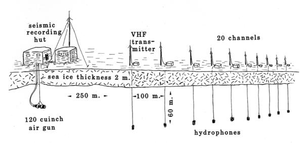
Fig. 5.1 Array of modified sonobuoys used for seismic multi-channel seismic reflection measurements on drifting sea ice. From Kristoffersen and Husebye (1985).
