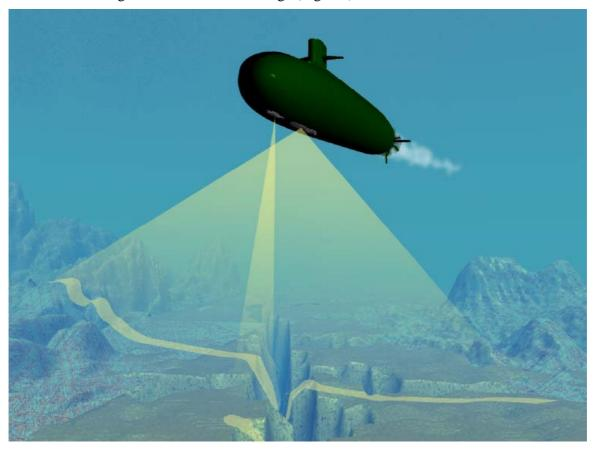
Fig. 4.7 The concept for seabed mapping and charaterization from a nuclear submarine platform as successfully carried out by U.S.N. Hawkbill in 1999 (Figure courtesy of Paul Bienhof).
