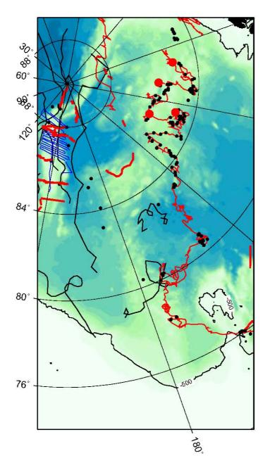
Figur 4.2 Plot of seismic reflection data collected from Alpha Ridge and its vicinity: icebreaker surveys (heavy red lines), drifting ice stations (thin black lines, Russian; thin red lines, Canadian and U.S.), and SCICEX high resolution chirp sonar surveys (thin blue lines). The seismic data was acquired by "Polarstern" in 1991 and 1998, "Oden" in 1996, Arlis-II in 1964-65, CESAR in 1983, T3 in 1966-74 and by Russian icestations NP-13, NP-21, NP-22, NP-23, NP-24, NP-26 and NP-28.
