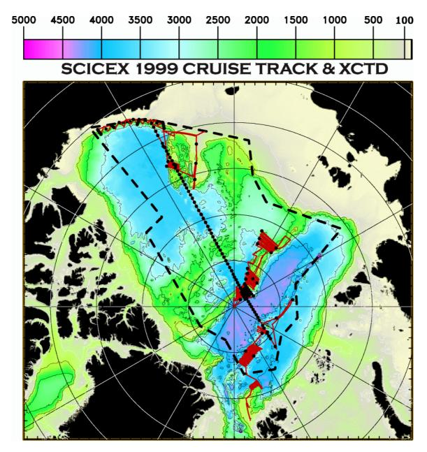
Fig. 4.8 SCICEX 1999 Cruise track with swath bathymetry and chirp sonar recording (red line). Black dots along the basin transect from Alaska towards Franz Josef Land indicate locations where expendable probes for sea water conductivity, temperature and depth (X CTD) were deployed. Approximate limit of 200 n.m. Exclusive Economic Zone indicated by dashed black line. Figure from : <u>http://boreas.coas.oregonstate.edu/scicex/scicexmaps/</u>
