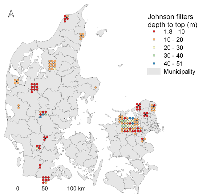
Figure 7-2: Depth to top screen (m below ground surface, m b.g.s) of the active GRUMO wells with Johnson filters. The filters are shown in a matrix around the cluster centre (black dot) to avoid overplotting. Bornholm is not shown as there are no Johnson filters there.
