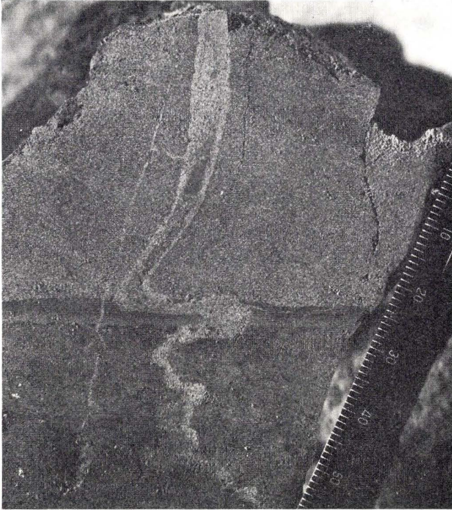
Text-fig. 4. Ptygmatic folding of an ashfilled fissure in the clay below +90. A thin layer of clayey sediment is seen between the two components of the double-layer.
