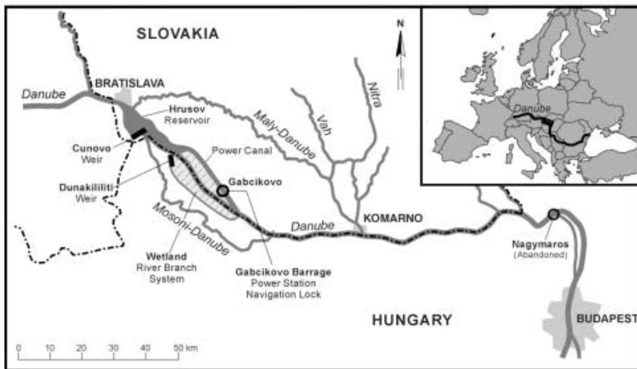
Fig. 20 The Danubian Lowland with the new reservoir and the Gabčíkovo hydropower scheme.
