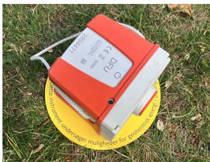
Figure 4: A Sercel WiNG DFU wireless node. The round yellow sign contains a short information to the public about the acquisition and a link to a project webpage.
