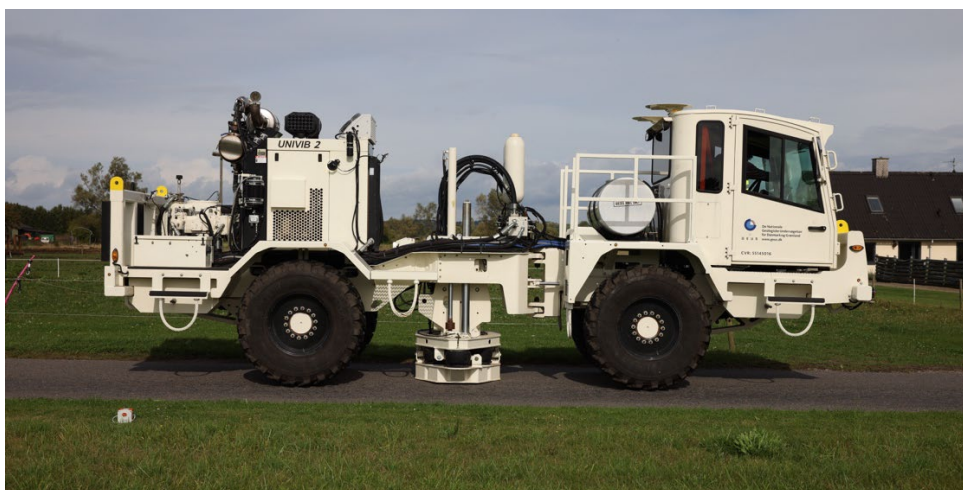
Figure 3: One of GEUS' 16.5 tonnes UV2 vibroseis truck form INOVA Geophysical.
