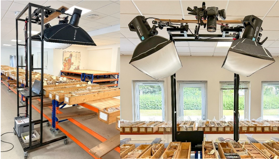
Figure 4 Photo setup of the GEUS Core Store mobile photo rig. During imaging, the windows are covered to minimize interference from outside light
