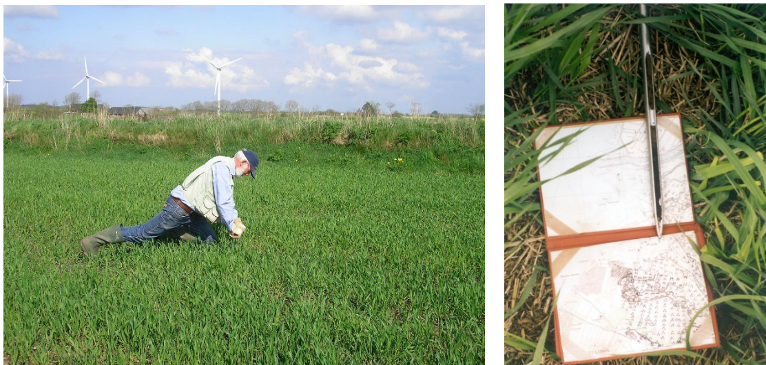
Figure 3. The 1-metre-long soil spear is pressed into the ground. The sample is situated in a groove at the tip of the soil spear. The soil type is determined on site, and the result is plotted on the field map.
