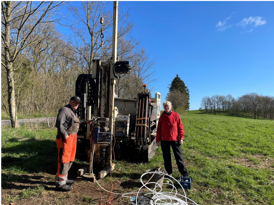
Figure 5. Drilling well V2, DGU. 49.2528, with med Geoprobe May 17 th , 2023, DGU. 49.2528
