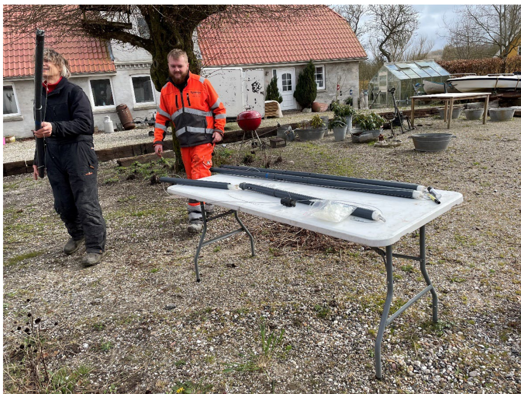
Figure 4. Sampling devices for depth specific sampling in existing wells with a long open borehole/intake in the chalk aquifer. May 1 st , 2023, DGU 49.386.
