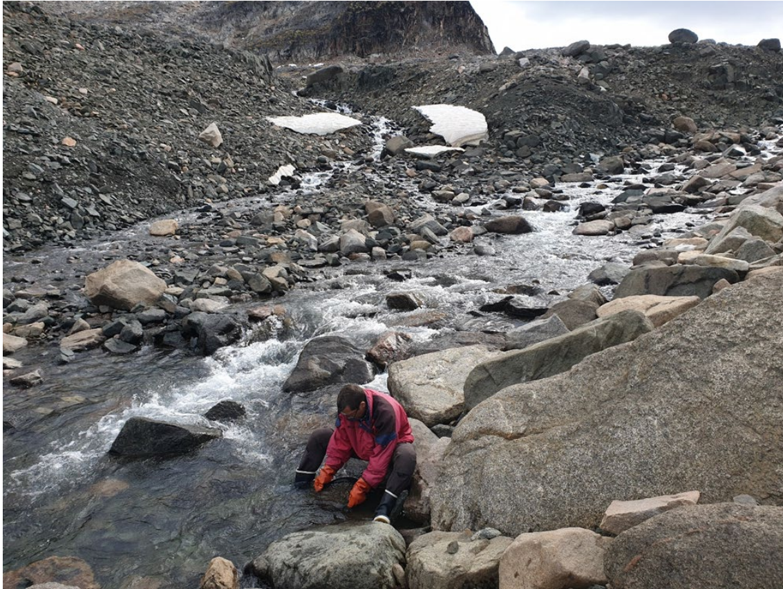
Figure 4. First stage of panning, to remove coarser rock fragments and part of the clays, before sieving.
