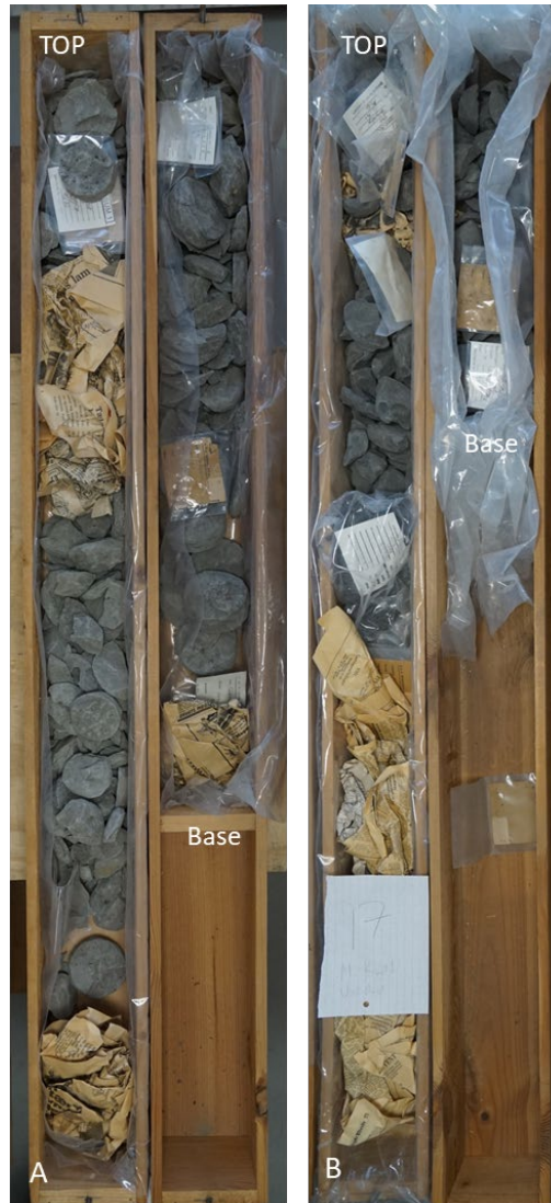
Figure 7.2.5 Core photos of the Vested Fm, Gassum-1 well. A. Lower Hauterivian, grey–dark grey calcareous mudstones Core 18, 3490–3501' (c. 1064–1067 m). B. Middle Barremian highly calcareous grey mudstones. Core 17, 3305–3325' (c. 1007–1013 m). Note the general poor core condition, core diameter 8.5 cm.
