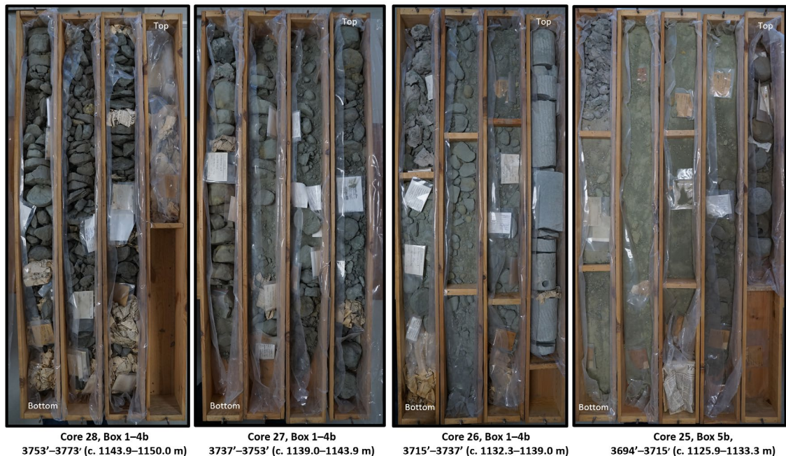
Figure 7.1.17. Core examples of the Frederikshavn Fm from the Gassum-1 well dominated by very fine-grained sandstones that are greenish grey in colour, probably due to a content of glauconite. In general, the cores are fragmented or even disintegrated, but more coherent (cemented) sections still exist. Given the state of preservation the cores may form a basis for studies of depositional environments, reservoir and seal properties including porosity, permeability, grain size, mineralogy, diagenesis. Core diameter is c. 8.5 cm.
