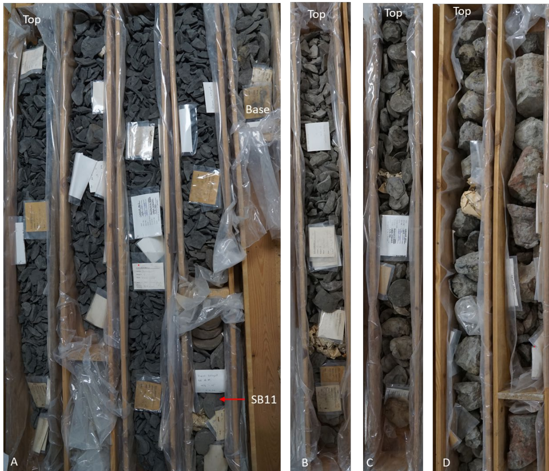
Figure 7.2.3. Core photos of the Fjerritslev Fm, Gassum-1 well. A. F-Ia mb, Hettangian–Sinemurian transition. The SB 11 is present in sandy grey mudstone in the lower part of the core and is overlain by very dark grey mudstones. Core 47, 4702–4722' (c.1433–1439 m), B. F-III mb, Pliensbachian. Grey bioturbated silty mudstone, sequence 14. Core 33, 4016–4021' (c.1224–1226 m) C. F-III mb, Toarcian. Grey bioturbated silty mudstone above SB 15. Core 32, 3967–3972' (c.1209–1211 m). D. Børglum Fm, Oxfordian–Kimmeridgian. Greenish grey and reddish mudstones indicating diagenetic overprinting due to subaerial weathering. Core 31, 3903–3914', (c.1190–1193 m). Note general poor core conditions, core diameter 8.5 cm. Core depths may differ from log depths, see Nielsen (2003, fig. 13).
