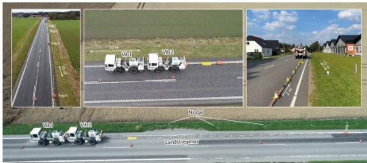
Figure 4.2.2 A series of field photos showing different parts of the dual element acquisition setup including 4–5 segments (each 20 units and 2 m spacing) MEMs based and nodal recorders (spaced at every 10 m) where shots were generated using two 12t mini vibrators.
