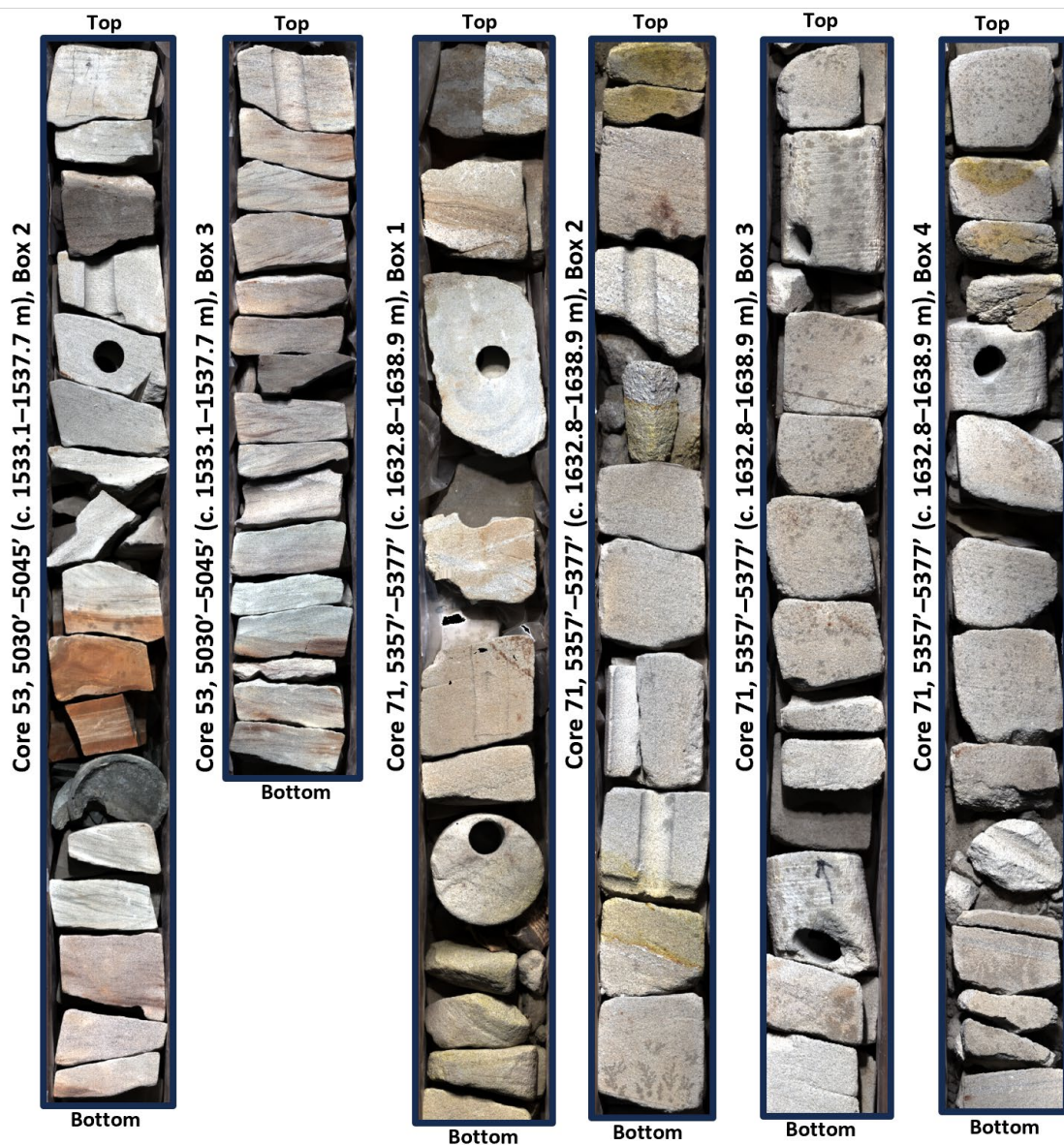
Figure 7.1.13. Cores of the Gassum Fm in the Gassum-1 well showing mainly fine- and medium-grained shoreface sandstones. Core diameter is c. 8.5 cm. Cored intervals are marked on the petrophysical log of the well in Fig. 7.1.2. Photos by Emil Fønss Jensen (Jensen 2023).
