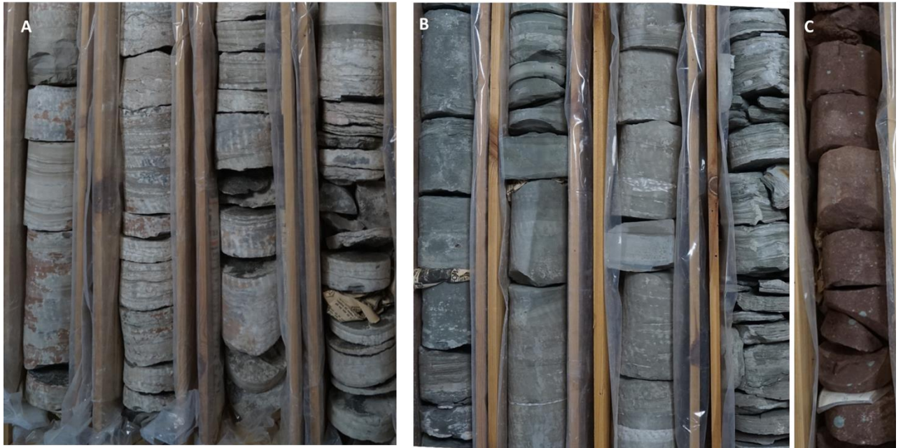
Figure 7.2.4. Photographs of the Ørslev Fm, Rødby-1 cores. A) Section from core 69, 3685'–3705' (1123–1129 m), Evaporite unit. Layered and nodular anhydrite, with occasional thin units of mudstones and sandstones. B) Section from core 67, 3612'–3628' (1101–1106 m), intermediate mudstone anhydrite unit of laminated greenish grey mudstones with few thin anhydrite layers, note desiccation crack to right. C) Section from core 65, 3480'–3485' (1061–1062 m), upper mudstone unit of reddish-brown mudstones and muddy sandstones with reduced greenish spots. Core diameter is 8.5 cm. Cored intervals are marked on the petrophysical log of the well in Figure 7.2.1.
