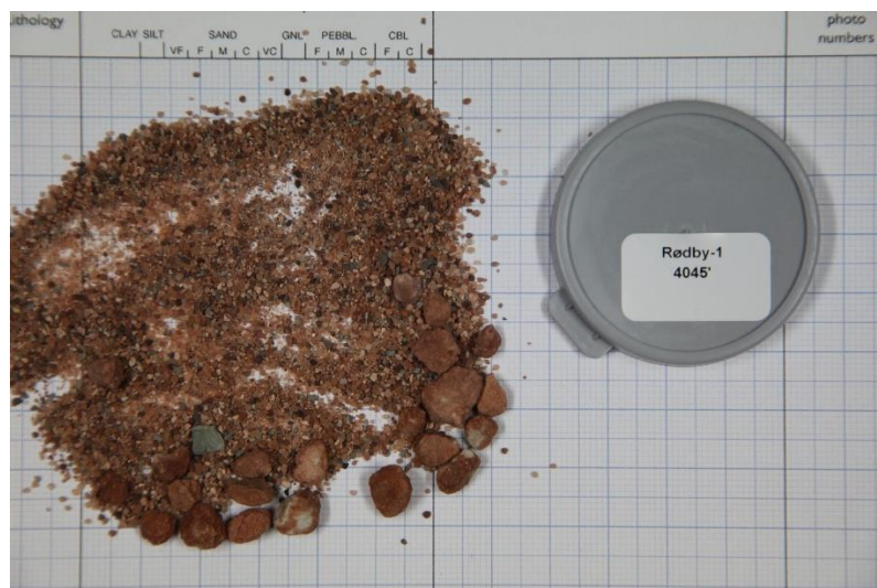
Figure 7.2.7 Photograph of a bulk cuttings sample from the Bunter Sandstone Fm at 1232 m (4045') below KB. The sample shows a dominance of quartz grains in the coarse sand fraction. The >5 mm grains in general consist of sandstones and claystones (DGU/DAPCO 1952). The sample also has a high Si content and a high Si/Al ratio, and an overall chemical composition
