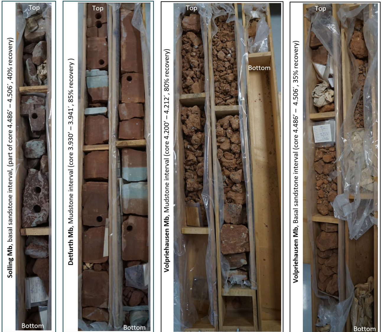
Figure 7.1.9. Cores of the Bunter Sandstone Fm in the Rødby-1 well showing the characteristic reddish-brown colour of the formation, however in places also with light greenish intervals or spots, probably reflecting local reducing conditions. Core diameter is c. 8.5 cm. Cored intervals are marked on the petrophysical log of the well in Figures 7.1.3 and 7.1.8.
