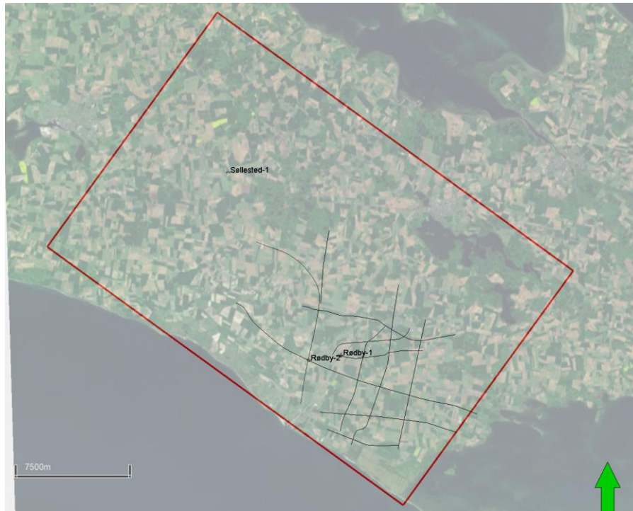
Figure 5.3 Area (28 by 18 km) of the regional velocity model, showing the used three wells, and the RMS migration velocities from the new GEUS2023-ROEDBY-RE2023 2D seismic lines (black lines).
