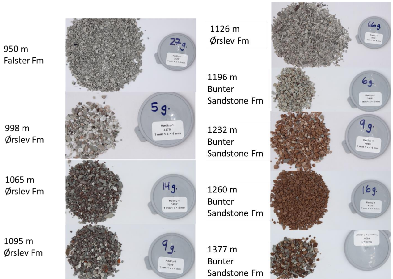
Figure 7.2.6 Selected pictures of cuttings in the 1–4 mm fraction from the Rødby-1 well. Grey lids shown to the right have a diameter of 45 mm. Depths are given in MD below KB. From Schovsbo & Petersen (2024).
