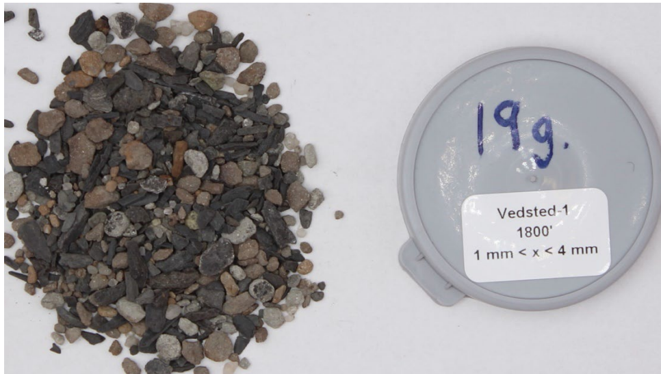
Figure 25 Cuttings from 1800 m (IMG_0992) in the Fjerritslev Formation, Vedsted-1 well. The sample has the highest Si/Al ratio in the Fjerritslev Formation and represents an interval with SP log readings that are markedly different the rest of the mudstone section. Grey lid shown to the right have a diameter of 45 mm. Note depth in meter (incorrectly shown as feet).
