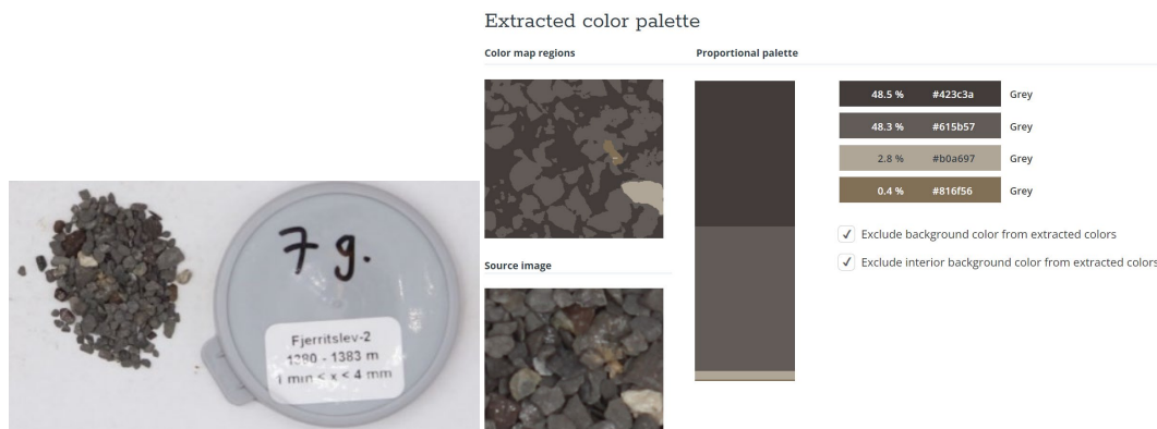
Figure 7 Example of analysis of image of the 1–4 mm cuttings fraction from 1380–1383 m in the Fjerritslev-2 well using TinEye Labs - Color Extraction Lab . The mudstone has two dominant grey colours. Less than 5 vol.% deviated from this and could potential reflect cavings or rare occurrence of rock types like concretions and/or sandy beds etc.
