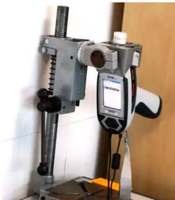
Figure 4 The Nithon XL3t GOLDD+ in a fixed analytical set-up at GEUS for measuring powdered samples.
