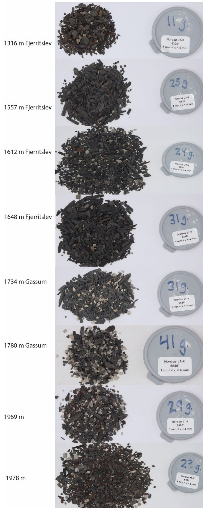
Figure 20 Selected images of the 1–4 mm cuttings fraction from the J-1X well. Grey lids with marked sample size in g shown to the right have a diameter of 45 mm.
