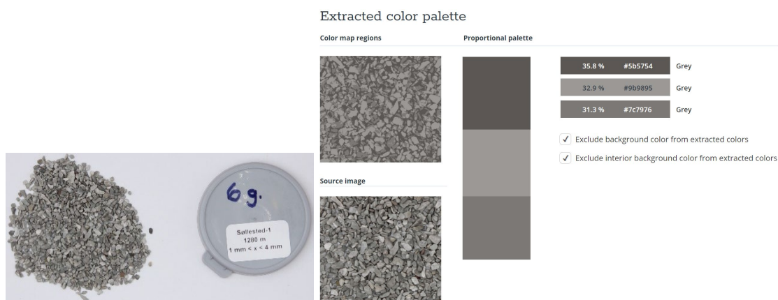
Figure 8 Example of analysis of image of the 1–4 mm cuttings fraction from 1280 m in the Søllestet-1 well using TinEye Labs - Color Extraction Lab . The sample appears to have three dominant grey coloured shaly rock types.
