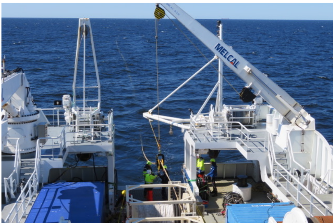
Figure 4. Recovery of the 2100-m-long streamer cable (Sercel Sentinel SSRD). Photo credit: Thomas Funck (GEUS).
