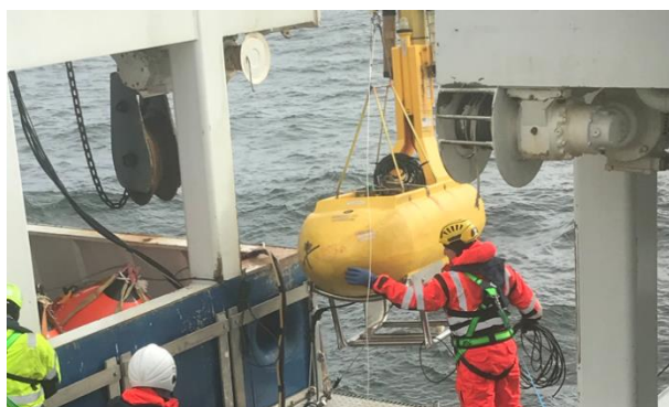
Figure 14 Deployment tail buoy
