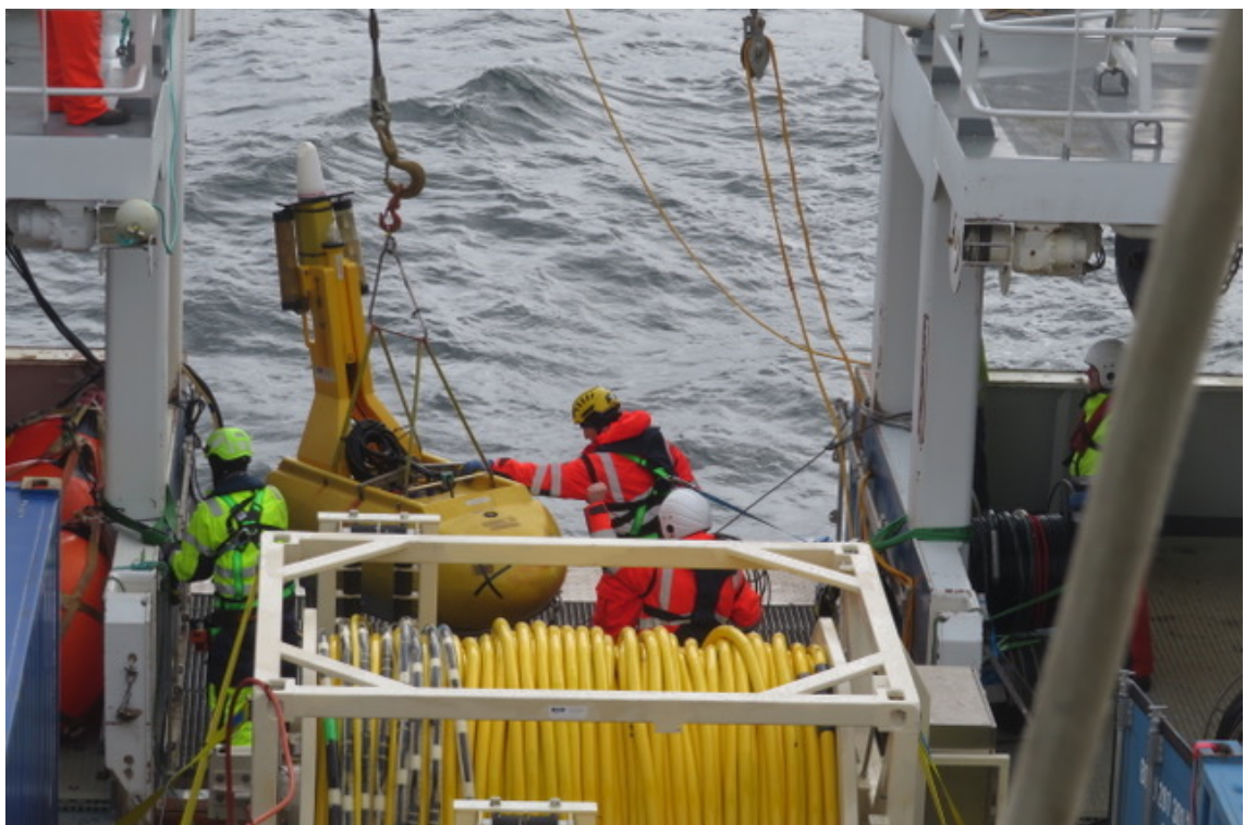
Figure 3. Deployment of the streamer tail buoy from the aft deck of Jákup Sverri . In the foreground one of the two winches for the solid-state streamer (Sercel Sentinel SSRD; yellow cable). Photo credit: Thomas Funck (GEUS).
