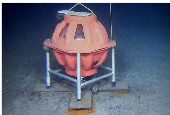
Fig. 4.2.5. Photo from Funck & Nørmark (2023) with an OBS (Sercel MicrOBS_Plus) attached to an anchor-cross on the seafloor.
