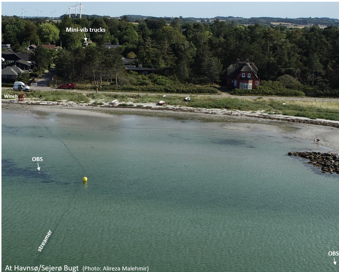
Fig. 4.2.6. Aerial view of the marine streamer and OBS. Onshore is the winch and in the background the approaching mini-vib trucks, which are the sources. Photo: Alireza Malehmir, 2022.
