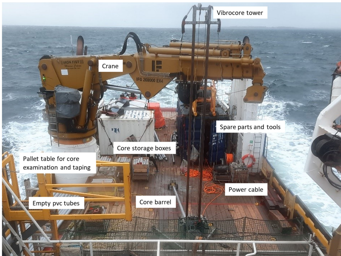
Figure 5.2 Deck arrangement of Fortuna Crane during vibrocore operations, looking aft from the bridge. Port side is to the right and starboard is to the left. The crane is mounted on the starboard side, but the vibrocrorer (centre of deck) is deployed over the port side.
