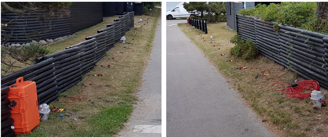
Figure 10. The short geophone cable with its geophones and the acquisition unit (orange box). The cable is coincident with some nodes (grey units) used in the main vibroseismic survey to verify the timing between the two independent acquisition systems.
