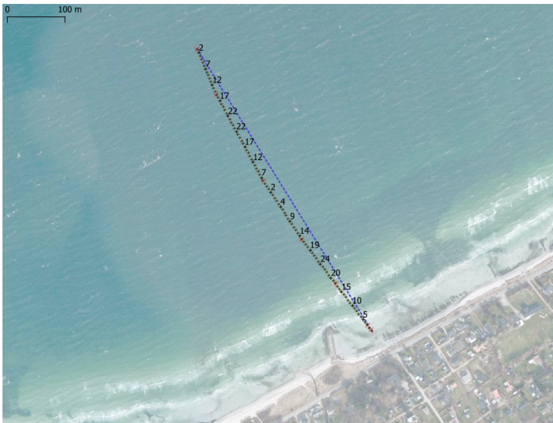
Figure 7. Interpolated positions of hydrophones. Original channel numbers are annotated.
