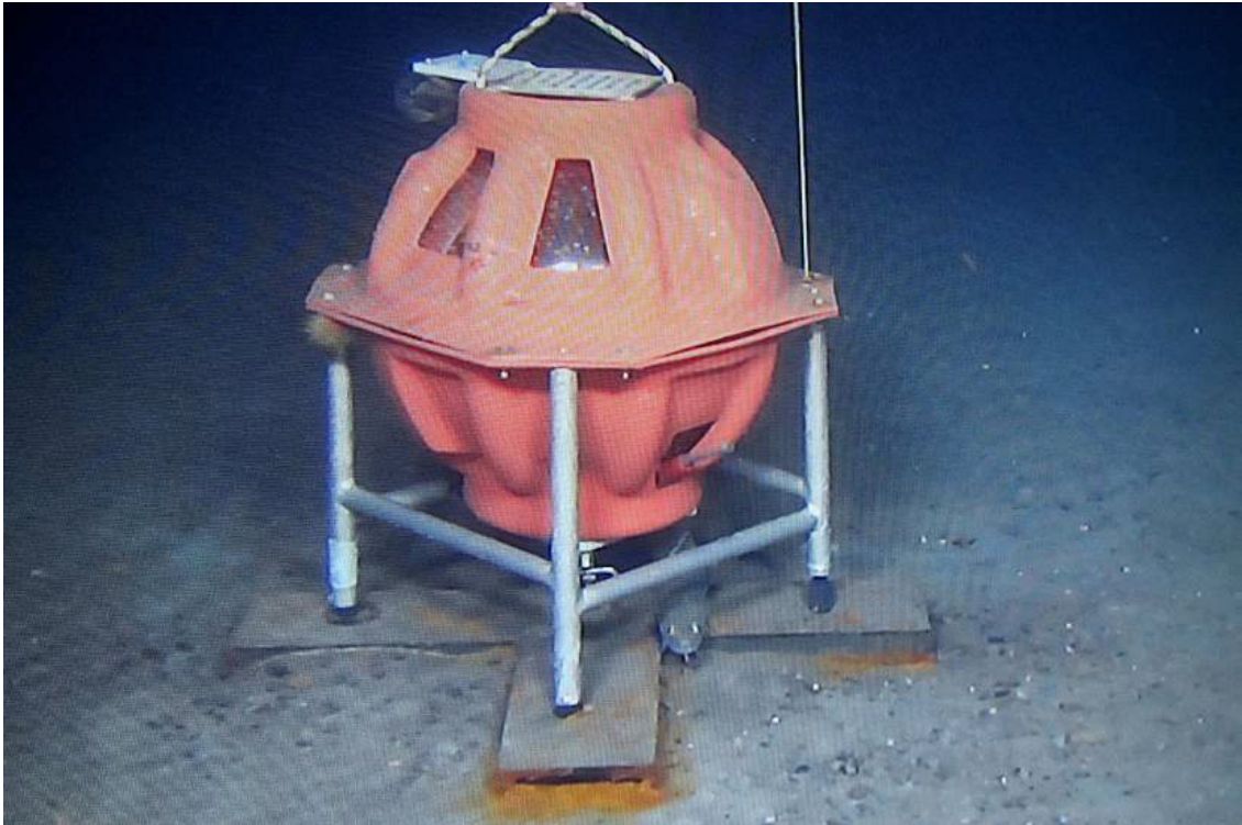
Figure 2. Sercel MicroOBS_Plus at the seafloor. The OBS is attached to an anchor (two crossing steel bars at the bottom) to allow for a good coupling of the geophones to the seafloor. Once the OBS is released from the anchor, it has enough buoyancy to return to the sea surface.
