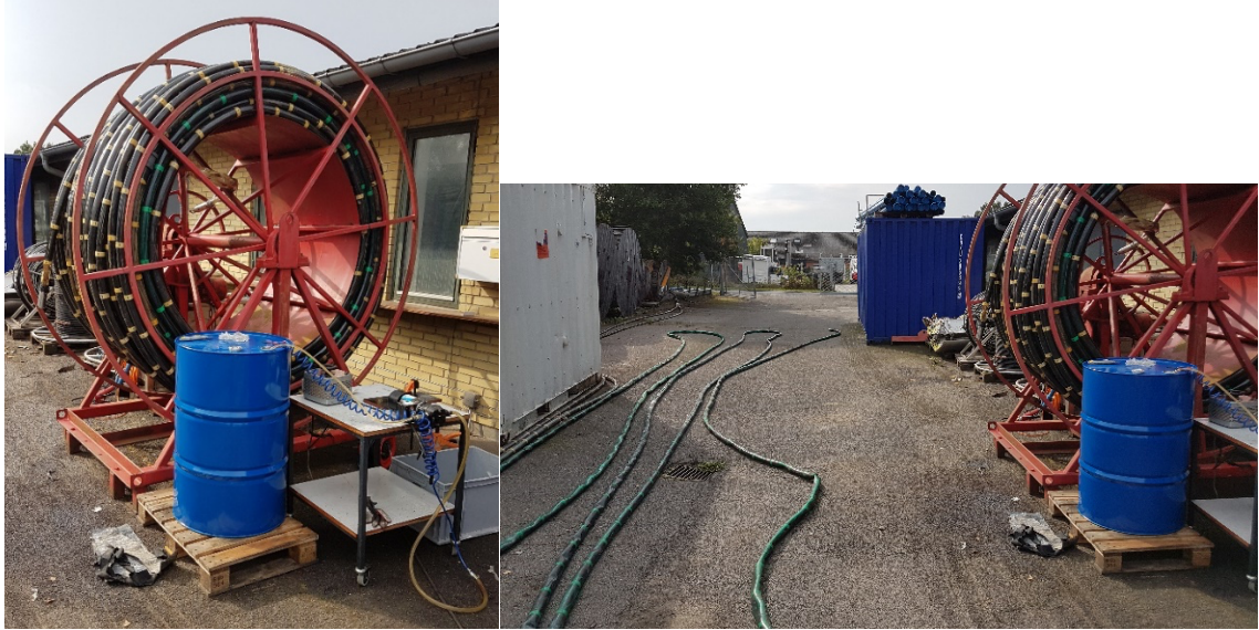
Figure 4. Refilling the streamer with kerosene.
