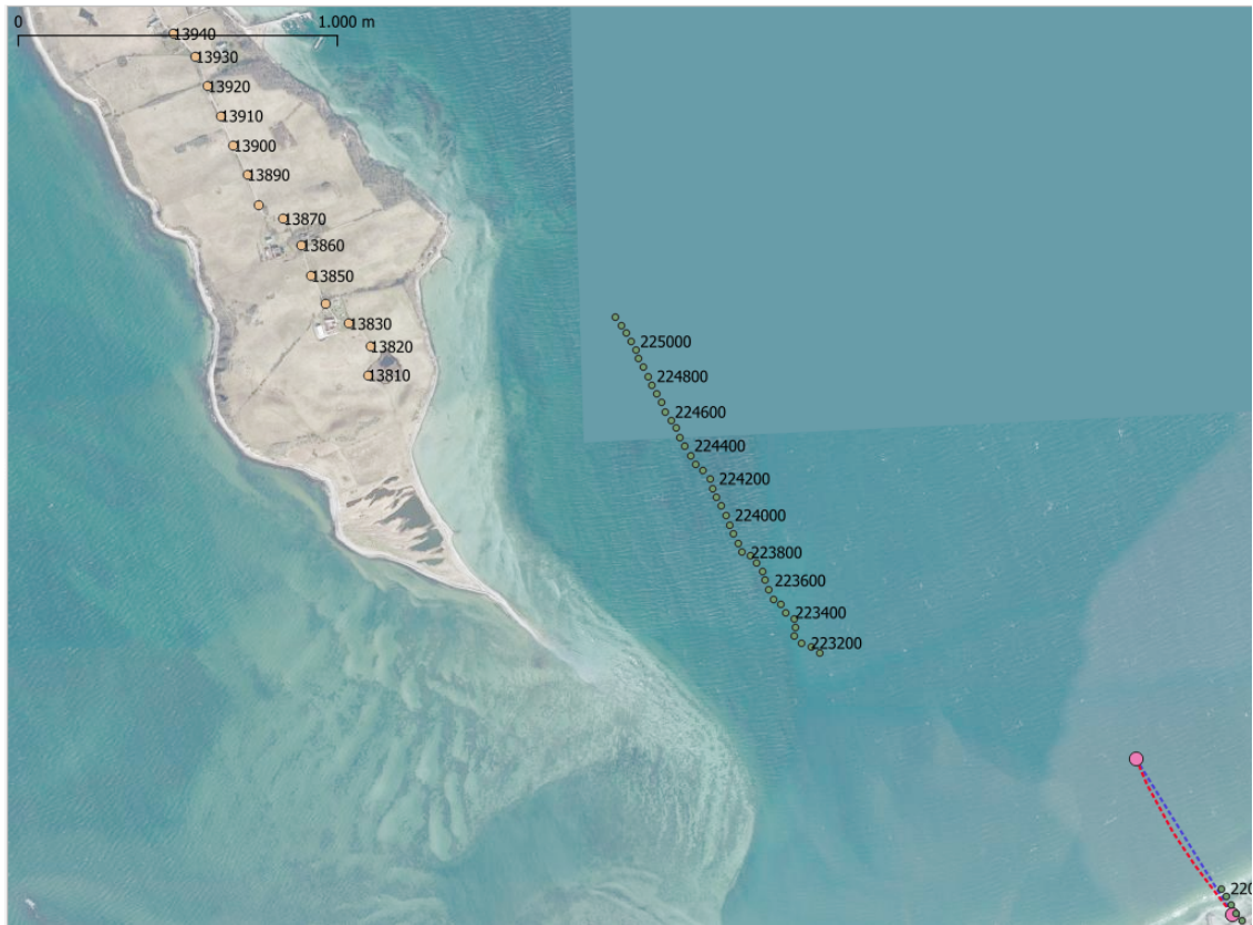
Figure 15. Vibration points on line GEUS22–HVN–P1 on the southern part of Nekselø are shown as orange circles (every 10 th point is shown). Vibration file numbers are annotated. CDP (common depth points) points for data acquired on the marine streamer from sweeps on Nekselø are indicated by green circles. CDP numbers are annotated.
