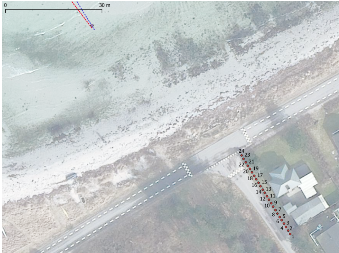
Figure 11. Position of geophones (red circles) used for the verification of the timing of the data. The near-shore part of the marine seismic streamer is seen top left. Channel numbers are annotated.
