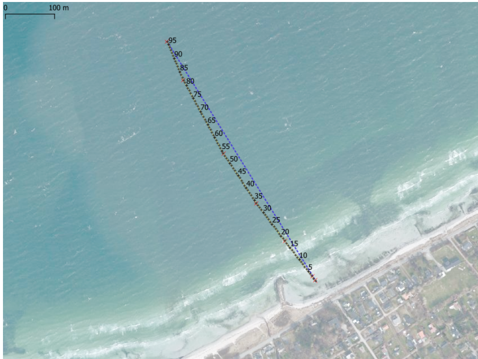
Figure 8. Interpolated positions of hydrophones. The renumbered channels are annotated.
