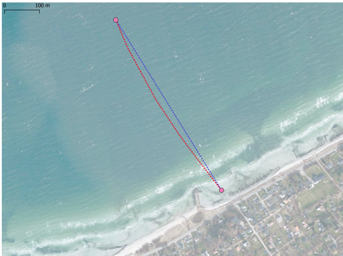
Figure 6. Blue line: straight line between the two endpoints of the streamer. Red line: the actual position of the streamer. Waypoints at the beginning and at the end of the streamer are marked by a red circle.
