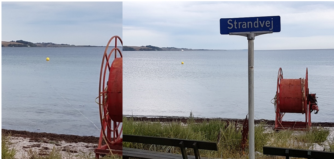
Figure 5. The streamer winch. The buoy attached to the near-shore OBS (station 15) is also seen.
