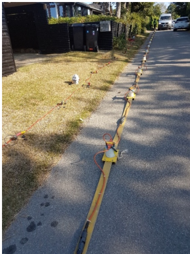
Figure 12. Left: short geophone cable (red cable in the grass) used to verify the timing of the signals. The land seismic streamer and nodes (on the pavement) and one of the wireless geophones (white box in the grass) used for the vibroseismic survey are also seen. Right: vibrator trucks at the closest vibration point to the shore.
