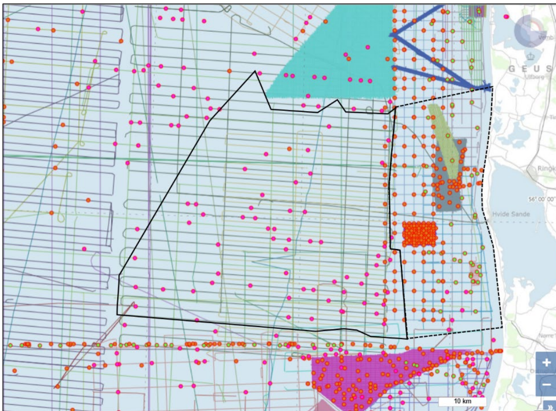
Figure 4.1. Shallow seismic lines and sediment core/grab sites in the screening area in the Danish North Sea (from GEUS' Marta database).
