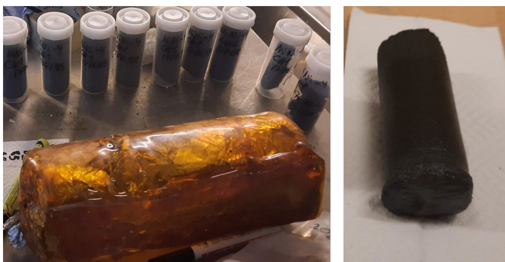
Figure 5 Seal peel of the core piece from the Nini-4 well (left). The cored plug was drilled from the seal peel, where oil can be seen saturating the plug (right).
