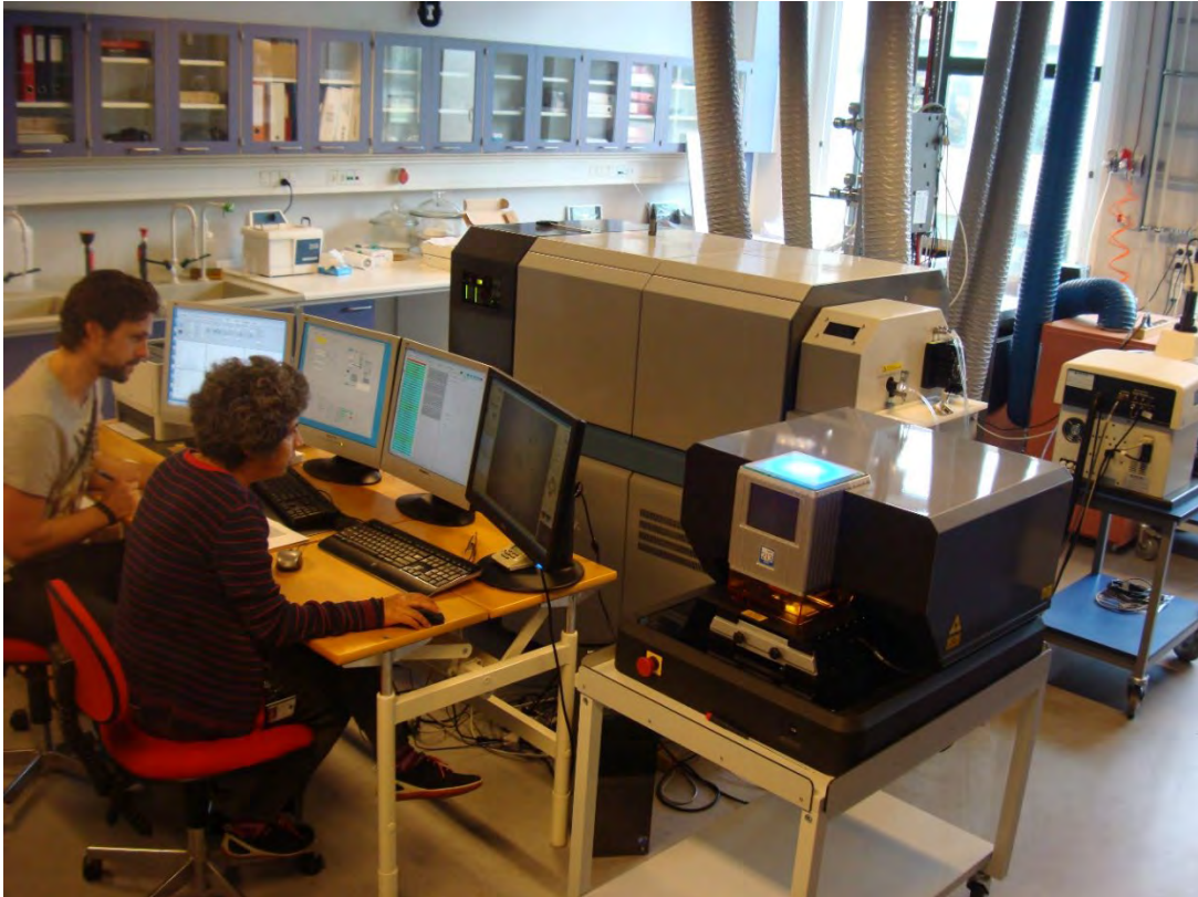
Figure 3: The Laser Ablation ICP-MS facility at GEUS (the laser ablation instrument in front).
