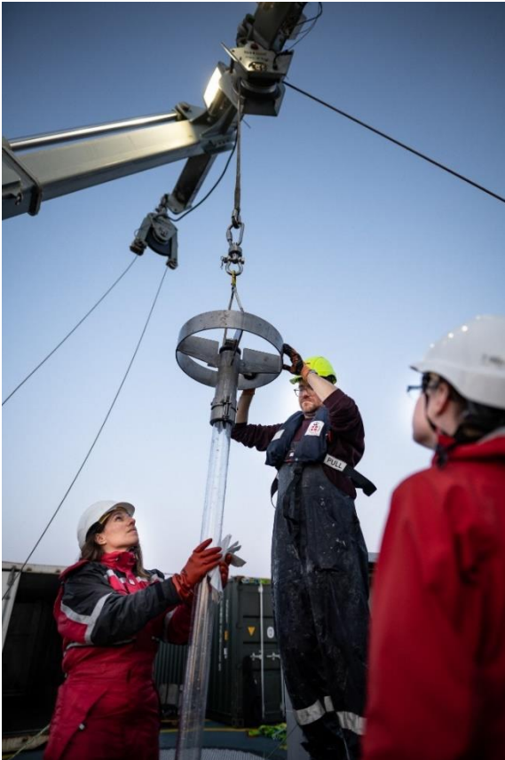
Figure 25 - Mounting of a liner in the Rumohr corer metal frame before deployment
