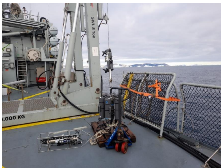
Figure 5- Complete Niskin-Rosette-CTD rack assembled for ICAROS 2021 in replacement for the planned SBE911 system.
