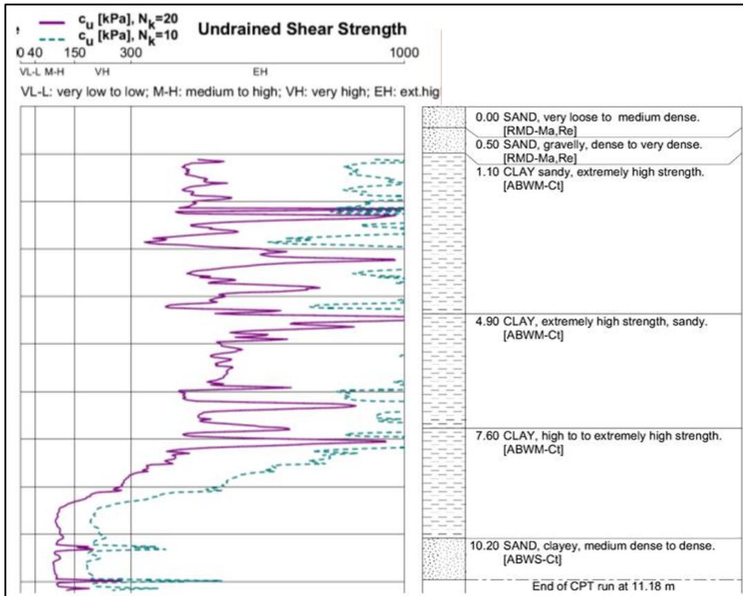
Figure 8.15 Undrained shear strength of RNB-CPT006 showing extremely high strength clay (till) to 10 m and medium high to high in the Bavneodde Greensand below (ref. Energinet 2014 (d)).
