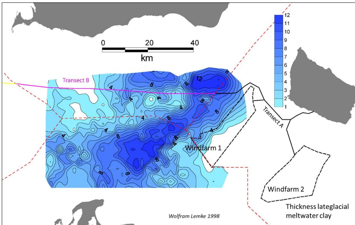
Figure 5.12 Thickness of Late Glacial clay mapped by Lemke (1998). The locations of Windfarm 1 and 2 (black dashed lines) and cable transects are indicated. The red dashed lines show the EEZ.
