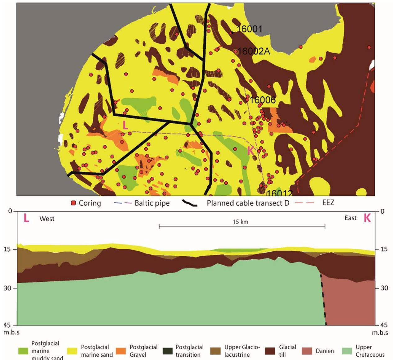
Figure 8.23 Upper figure: Surface sediments in the transect D Køge Bugt region. Location of Baltic Pipe profile section K–L is indicated. Lower figure: Baltic Pipe profile K–L interpreted sediment profile. For details see Appendix H.
