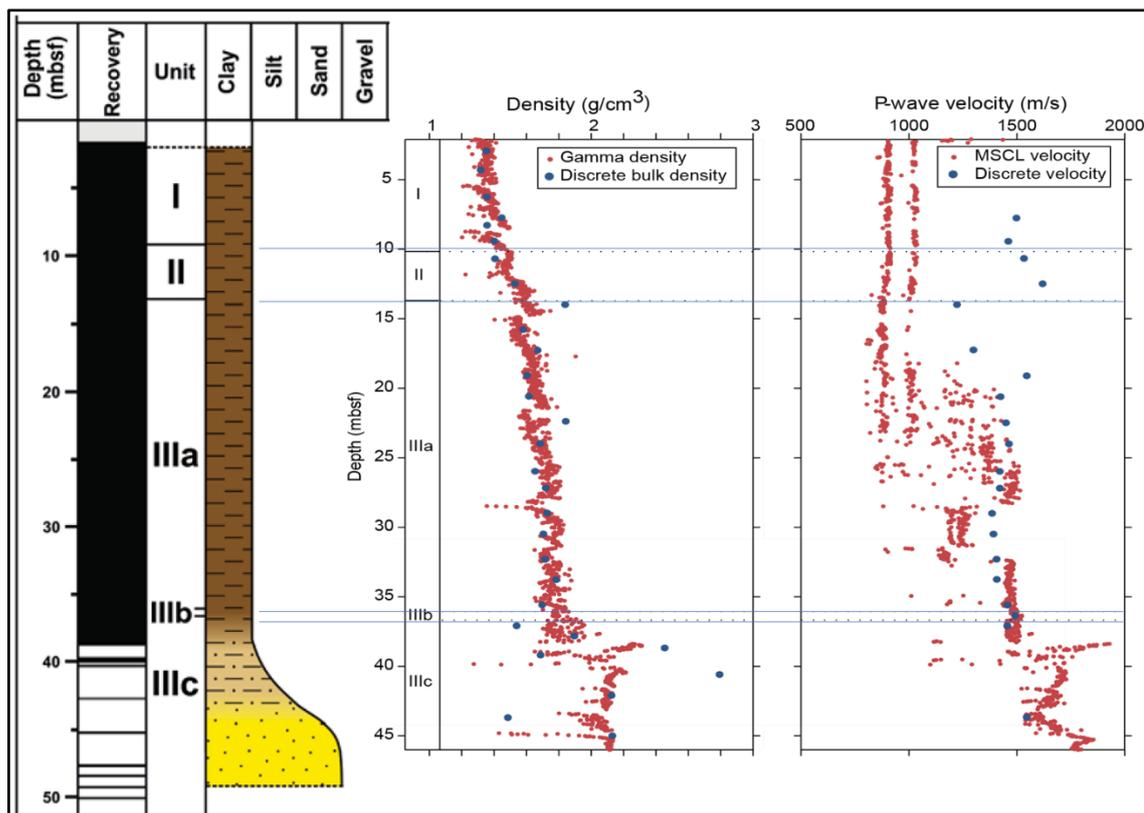
Figure 5.7. IODP Site M0065 core lithology, density and P-wave velocity.
