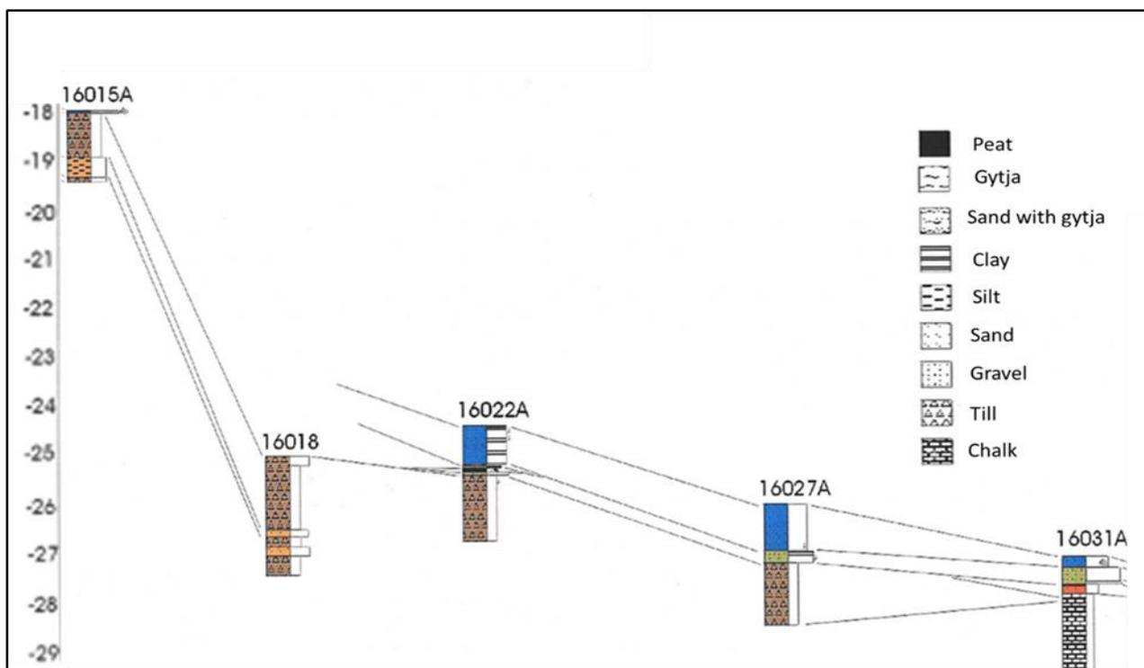
Figure 8.25 Vibrocore verification of surface-near sediments along profile M–N in Fakse Bugt (Figure 8.24 and Appendix I)
