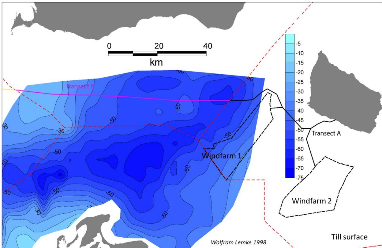
Figure 5.11 Till surface morphology mapped by Lemke (1998). The locations of Windfarm 1 and 2 (black dashed lines) and cable transects are indicated. The red dashed lines show the EEZ.
