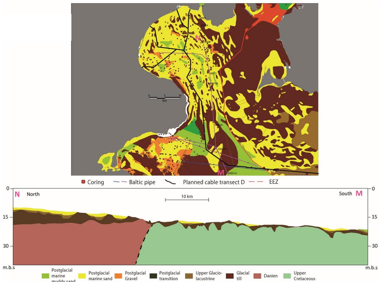
Figure 8.24 Upper figure: Surface sediments in the transect D Køge Bugt region. The location of Baltic Pipe profile section M–N is indicated. Lower figure: Baltic Pipe profile M–N interpreted sediment profile. For details see Appendix I.
