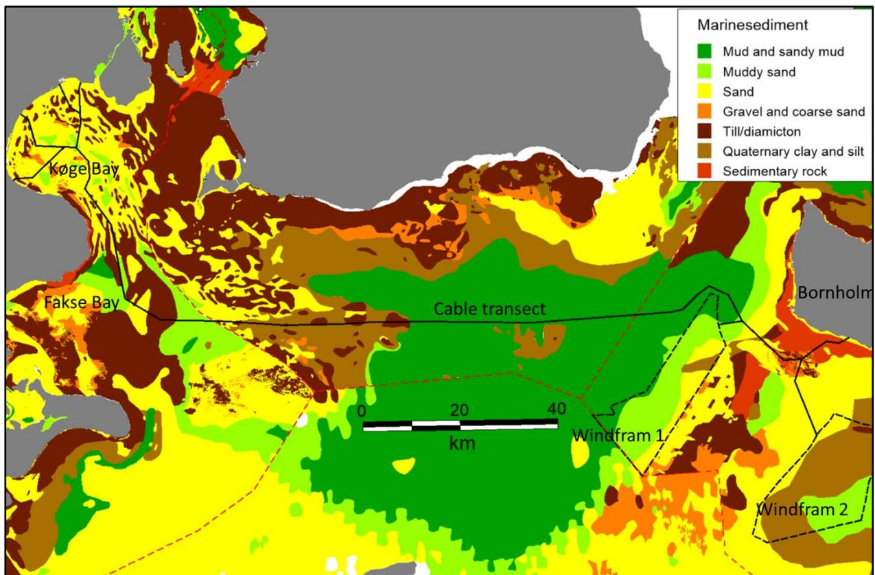
Figure 6.1 Seabed substrate map from the cable transect area based on a combination of Emodnet 1:1 M and Danish 1:100,000 2020 version.
