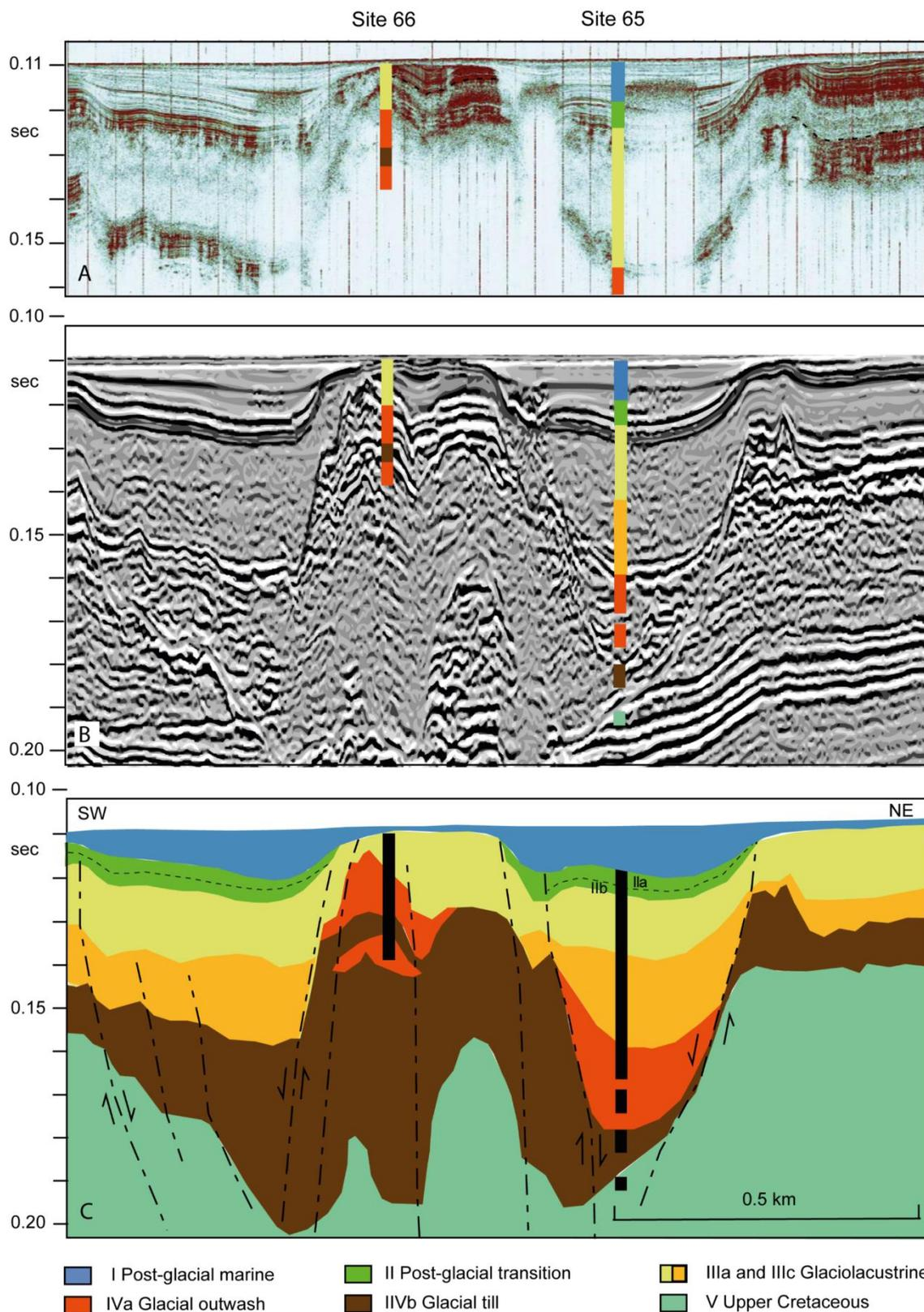
Figure 5.5. Seismic profiles across site M0065 and M0066 (Jensen et al.2017). Original interpretation of the seismic transect: Airgun (A) and Atlas parasound (B) data (Andr en 2014), as well as sediment documentation for sites 65 and 66. The interpretation (C) follows the classification in seismic units described in Figure 5.4. The location of the IODP sites is shown in Figure 5.3.
