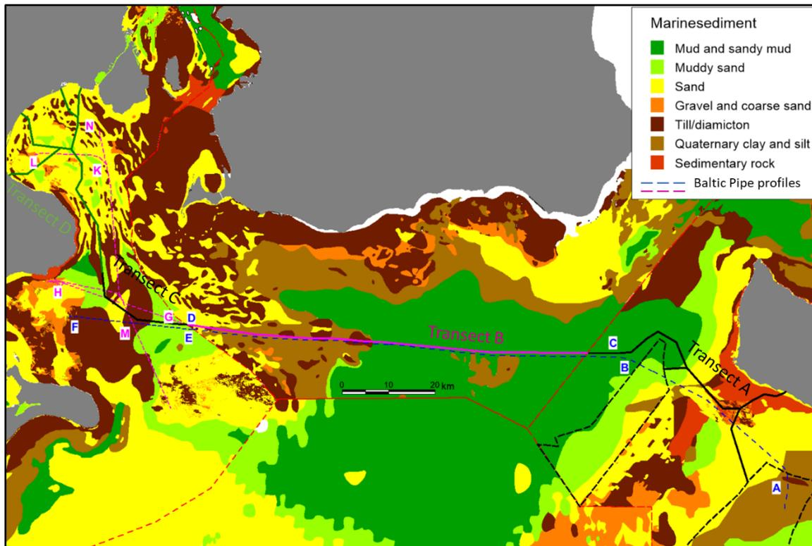
Figure 8.1 Seabed substrate map from the cable transect area base on a combination of Emodnet 1:1M and Danish 1:100,000 2020 version. Transects A–D is indicated as well as profile sections A–M. For details see Appendix B.
