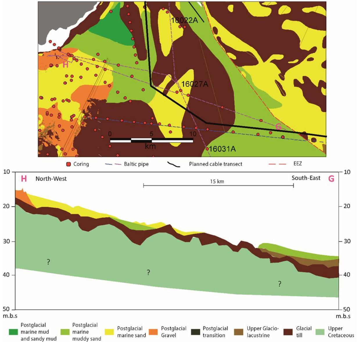
Figure 8.20 Upper figure: Surface sediments in the transect C outer Fakse Bugt region. The location of Baltic Pipe profile section G–H is indicated. Lower figure: Baltic Pipe profile G–H interpreted sediment profile. For details see Appendix F.
