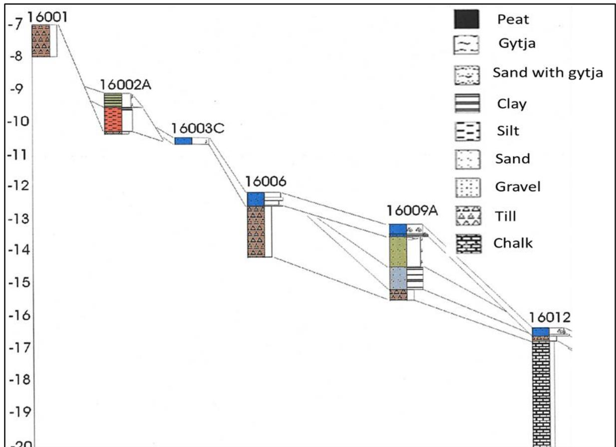
Figure 8.26 Vibrocore verification of surface-near sediments along profile M-N in Køge Bugt (Figure 8.24 and Appendix I).
