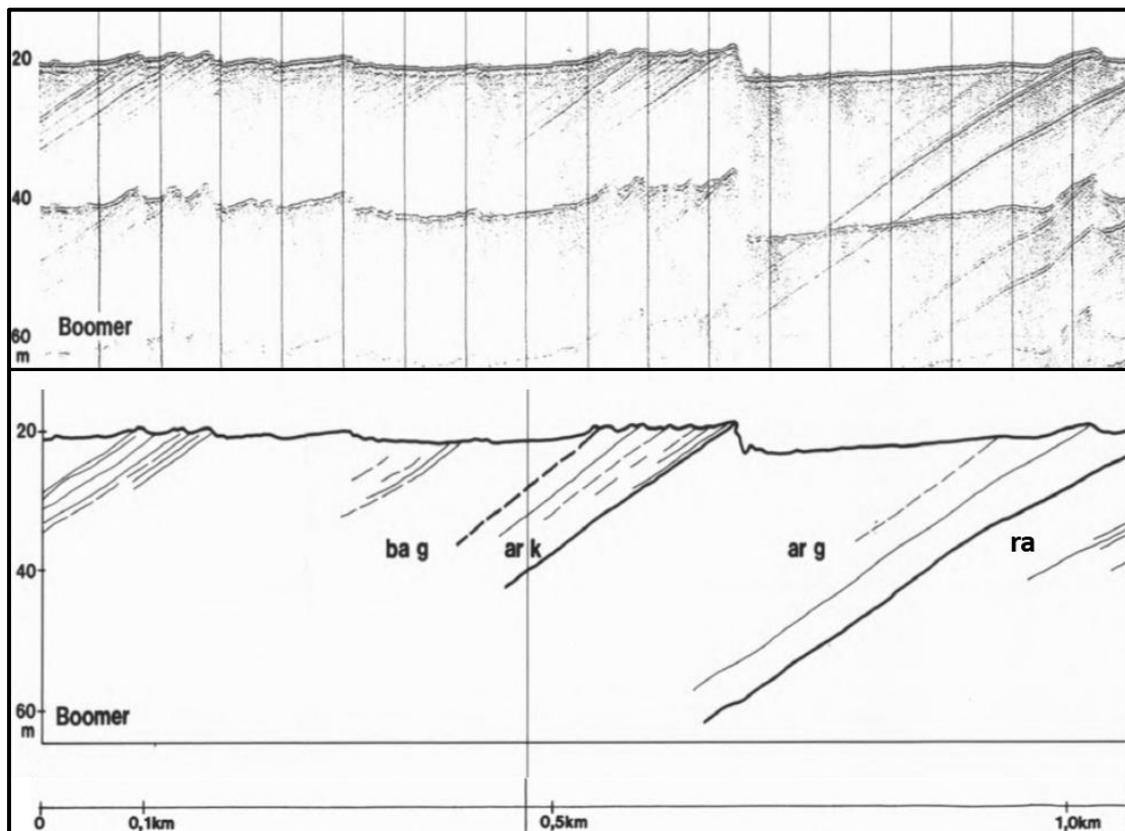
Figure 8.7 Boomer profile from the Rønne Graben illustrating the seismic reflection patterns of Rabekke Formation (ra), Arnager Greensand (ar g), Arnager Limestone (ar k) and Bagneodde Greensand (ba g).
