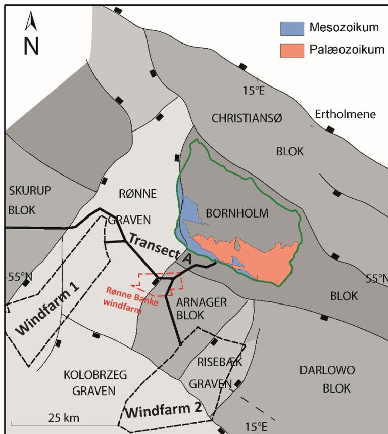
Figure 8.8 Major fault blocks of the Bornholm region. The fault pattern is based on Vejrbæk & Britze (1994) and Vejrbæk (1997). Location of Transect A, Windfarm 1 and 2 as well as Rønne Banke windfarm is indicated.
