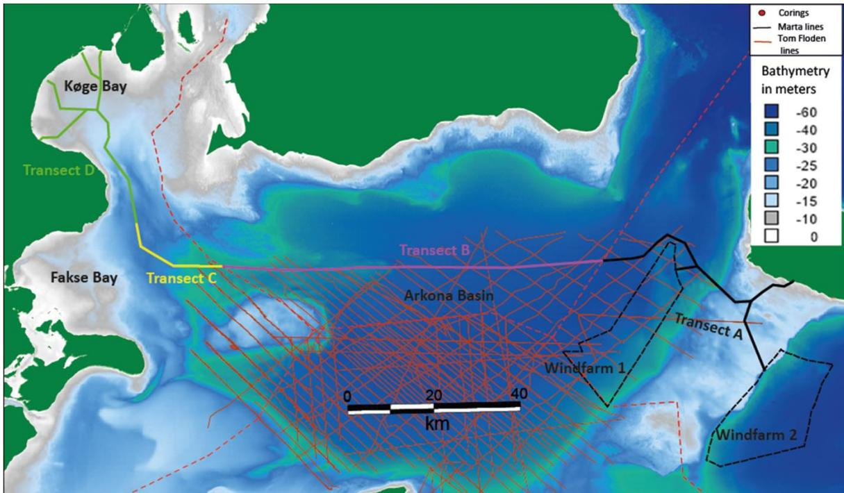
Figure 3.2 Archive seismic data collected by Tom Flodén from Stockholm's University used for general mapping in Arkona Basin by Lemke (1998). The locations of the proposed Windfarms are indicated by polygons. The bathymetry is from Emodnet.
