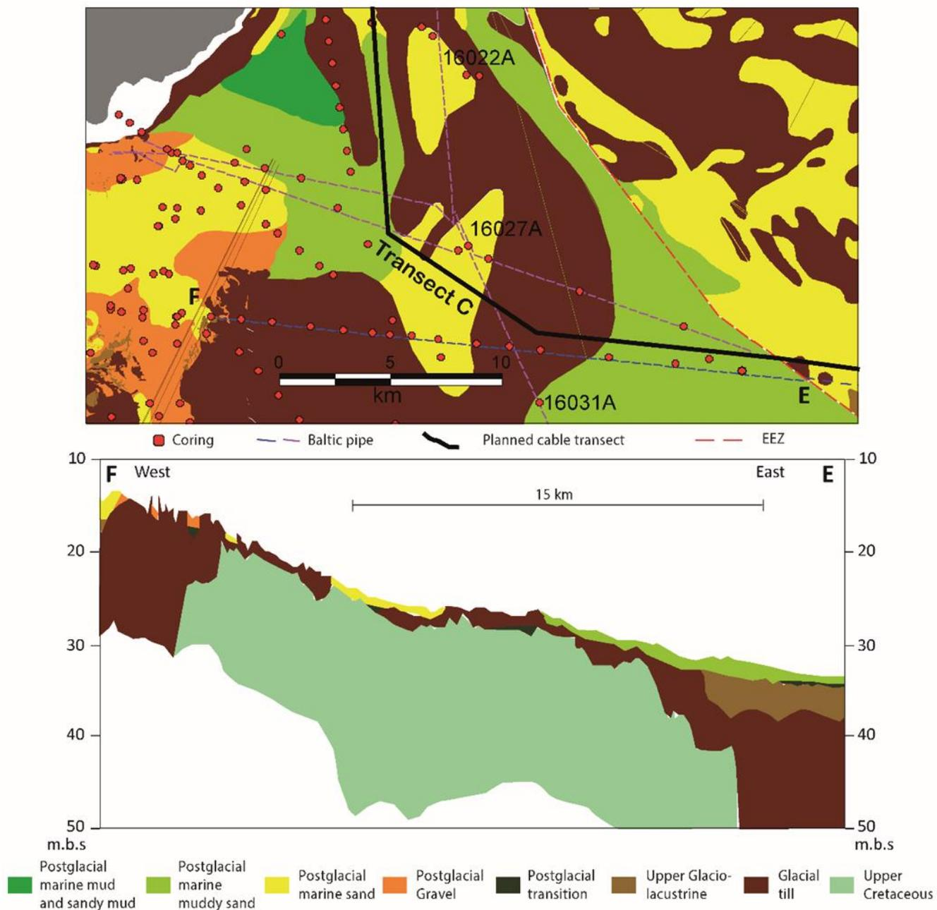
Figure 8.19 Upper figure: Surface sediments in the transect C outer Fakse Bugt region. Location of Baltic Pipe profile section E–F is indicated. Lower figure: Baltic Pipe profile E–F interpreted sediment profile. For details see Appendix E.
