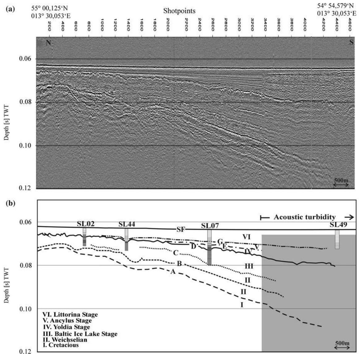
Figure 5.10 (a) Original seismic profile 21 with indication of an acoustic turbidity zone; (b) Seismostratigraphic interpretation of profile 21, SF = seafloor from Mathys et al. (2005). For location see Figure 5.3.
