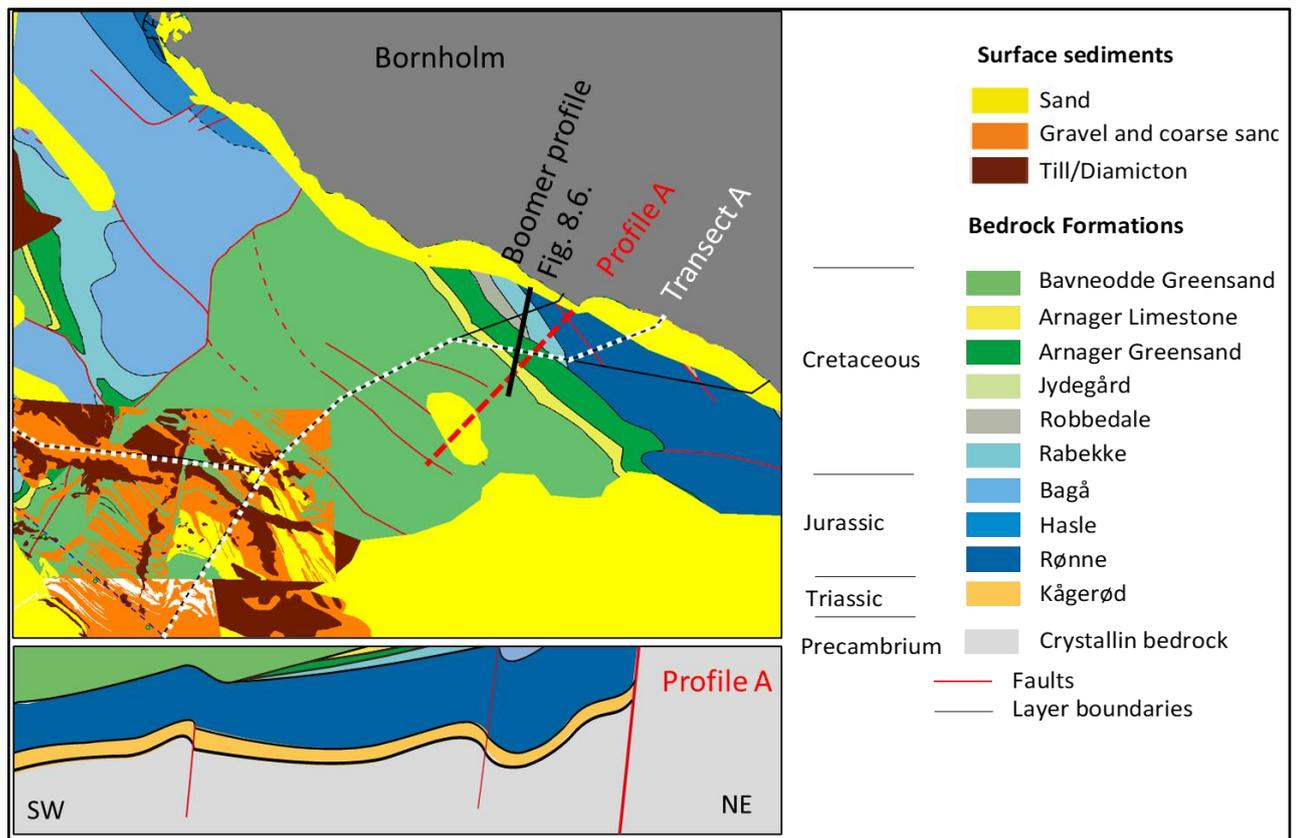
Figure 8.4 Near Bornholm surface sediments from Rønne Banke windfarm area, to Sose Bugt landfall, with pre-Quaternary seabed sediments barely covered by Quaternary sediments. Location of Boomer profile
