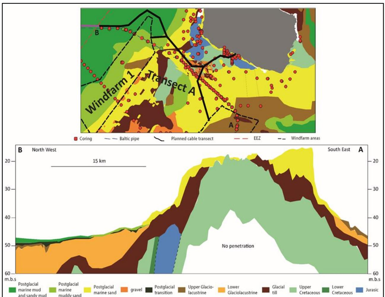
Figure 8.3 Upper figure: Surface sediments in the transect A region. Location of profile section A–B is indicated as well as locations of Windfarm 1 and 2 and vibrocore positions. Lower figure: Baltic Pipe profile A–B interpreted sediment profile. For details see Appendix C.
