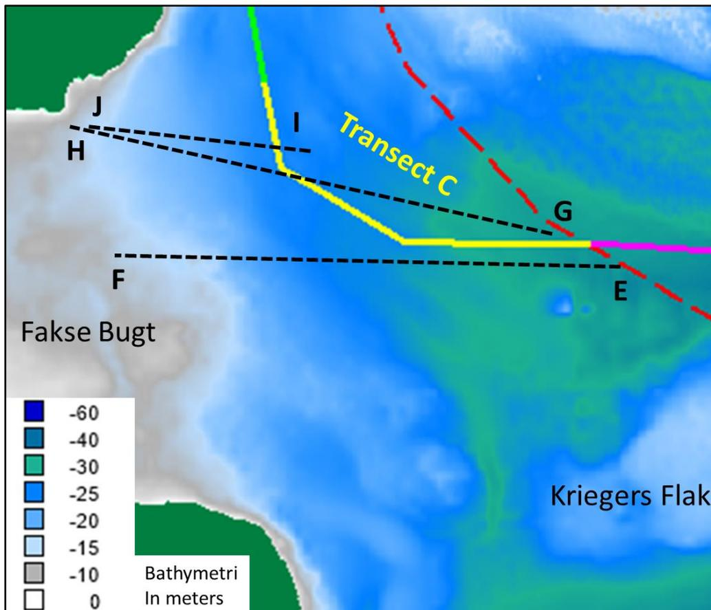
Figure 8.18 Bathymetry in the transect C area. The locations of Baltic Pipe profiles sections E–F, G–H and I–J are indicated.
