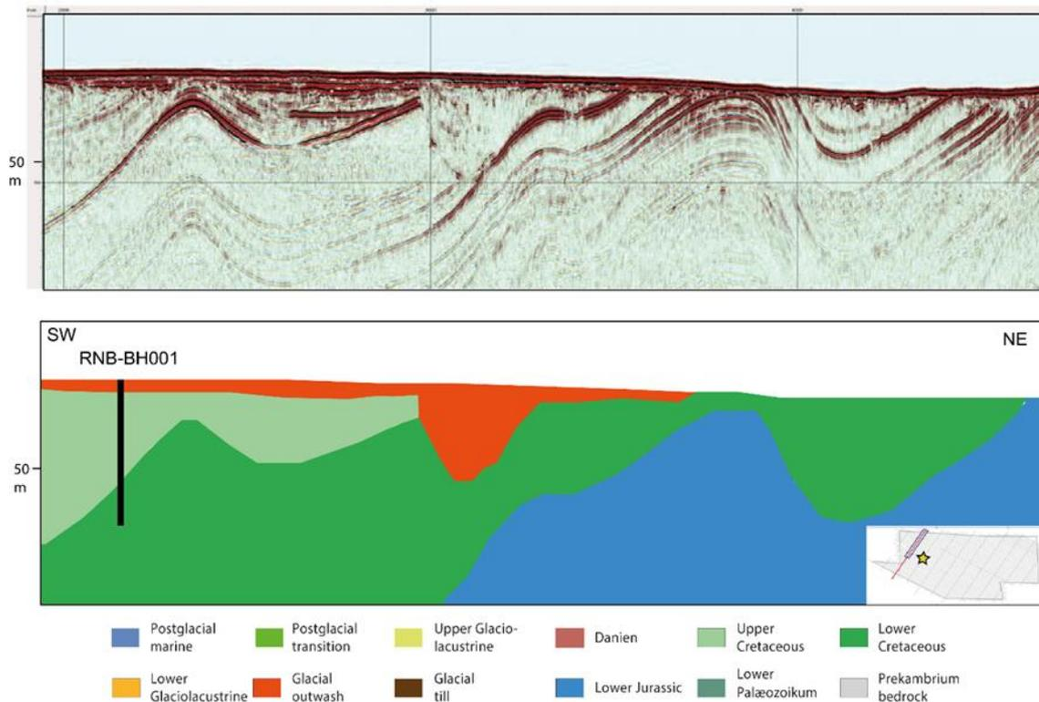
Figure 8.10 High resolution Sparker multi-channel profile XL\_010 and below geological interpretation. The location is indicated on the inset map in lower right corner.
