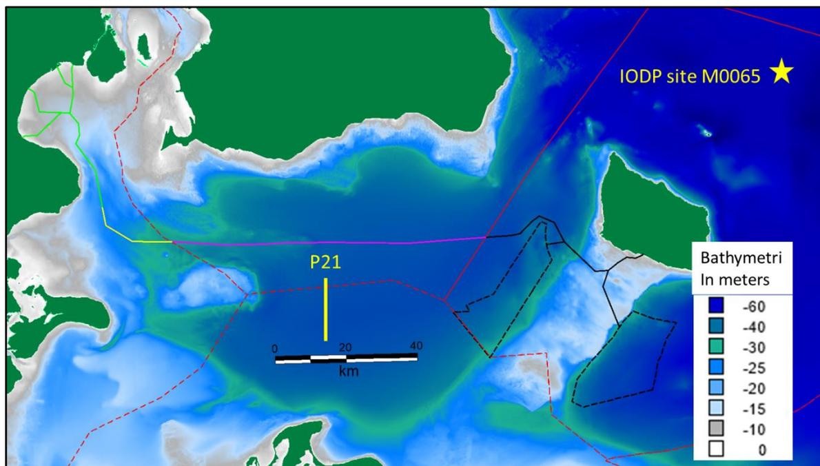
Figure 5.3. Map of the south-western Baltic Sea with location of IODP site M0065 (yellow star) in relation to the Windfarm 1 and 2 (polygons shown with black dashed lines) and cable lines. P21 shows the location of seismic line from Mathys et al. (2005). Red dashed lines: EEZ border.
