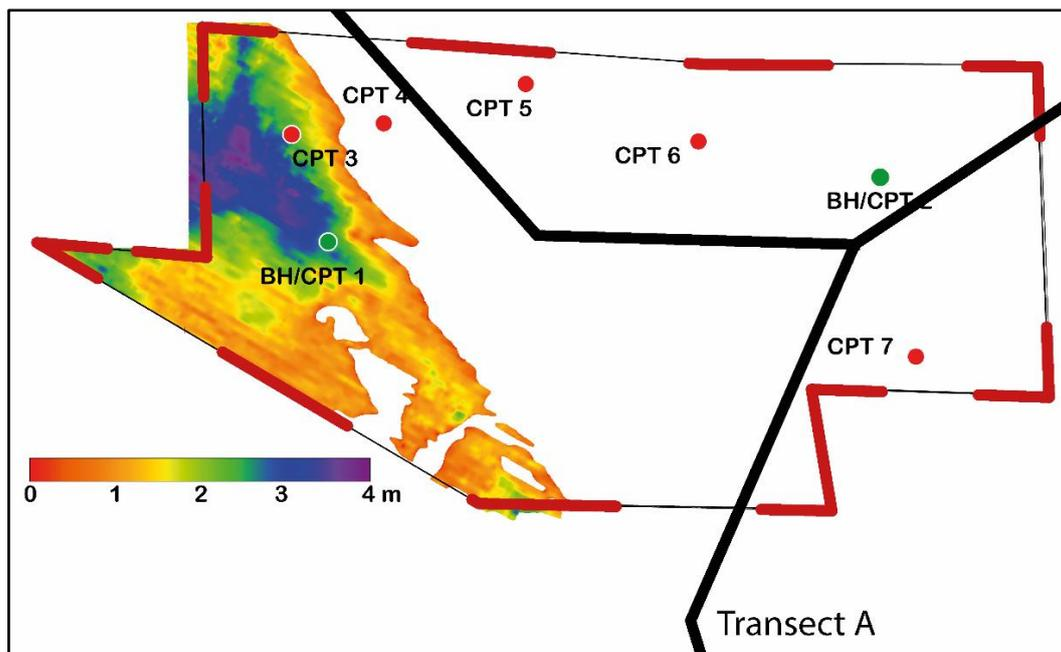
Figure 8.13 Thickness of Holocene marine deposits mapped from chirp seismic data. Locations of Transect A, Boreholes and CPT's are indicated
