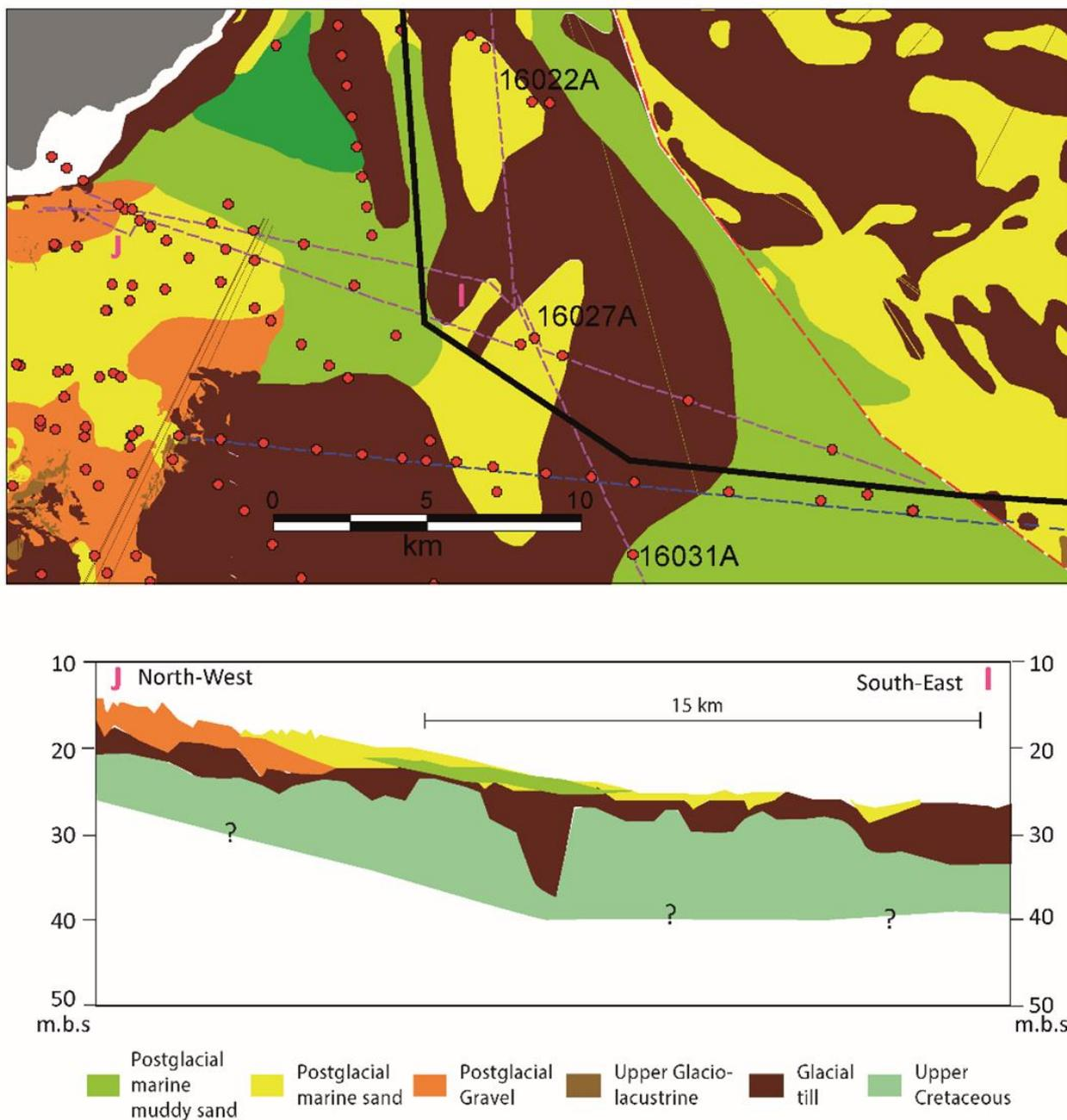
Figure 8.21 Upper figure: Surface sediments in the transect C outer Fakse Bugt region. Location of Baltic Pipe profile section I–J is indicated. Lower figure: Baltic Pipe profile I–J interpreted sediment profile. For details see Appendix G.
