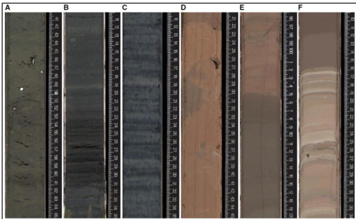
Figure 5.6. Examples of lithostratigraphic units, Hole M0065A. A. Unit I. B. Unit I. C. Unit II. D. Subunit IIIc. E. Subunit IIIb. F. Subunit IIIa.
