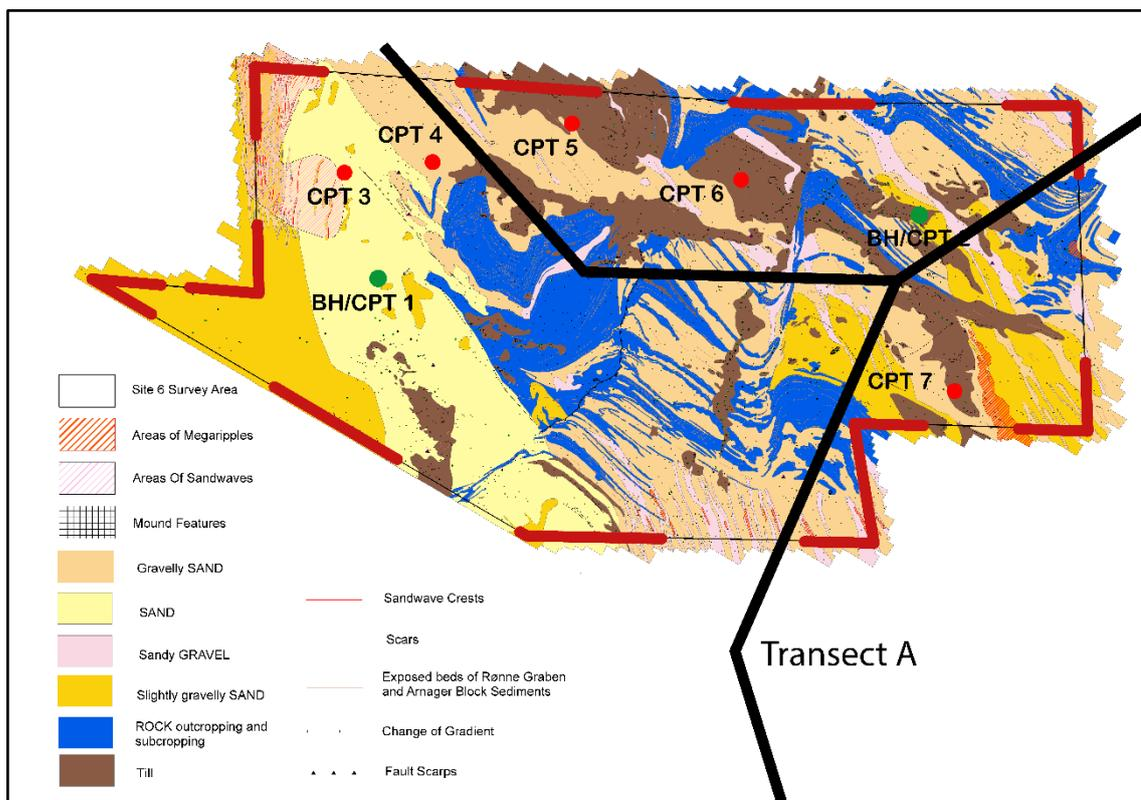
Figure 8.11 Seabed sediment map Rønne Banke Site 6. Surface sediment types and features are indicated as well as the locations of Transect A and boreholes (BH 1 and BH 2) and CPT's (CPT 1 to CPT 7)
