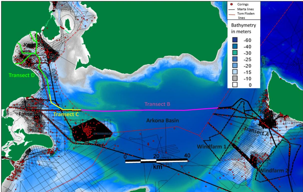
Figure 3.1. Distribution of Marta database seismic grid and core data southwest of Bornholm. The locations of the proposed windfarms are indicated by polygons. The bathymetry is from Emodnet.
