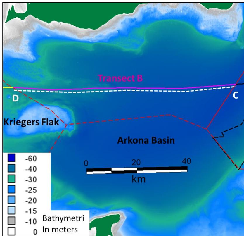
Figure 8.16 Bathymetry in the transect B area. The location of Baltic Pipe profile section C–D is indicated with a dashed white line.
