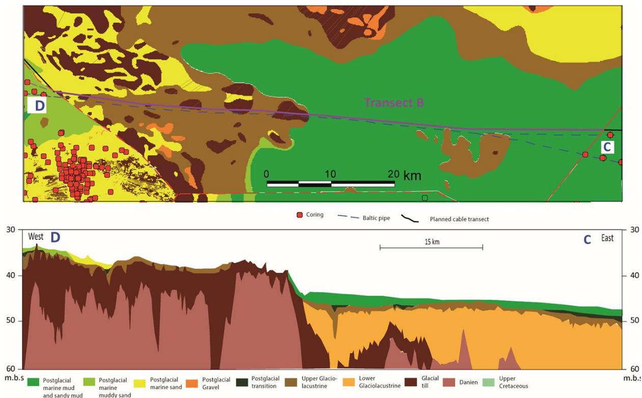
Figure 8.17 Upper figure: Surface sediments in the transect B Arkona Basin region. Location of Baltic Pipe profile section C–D is indicated. Lower figure: Baltic Pipe profile C–D interpreted sediment profile. For details see Appendix D.
