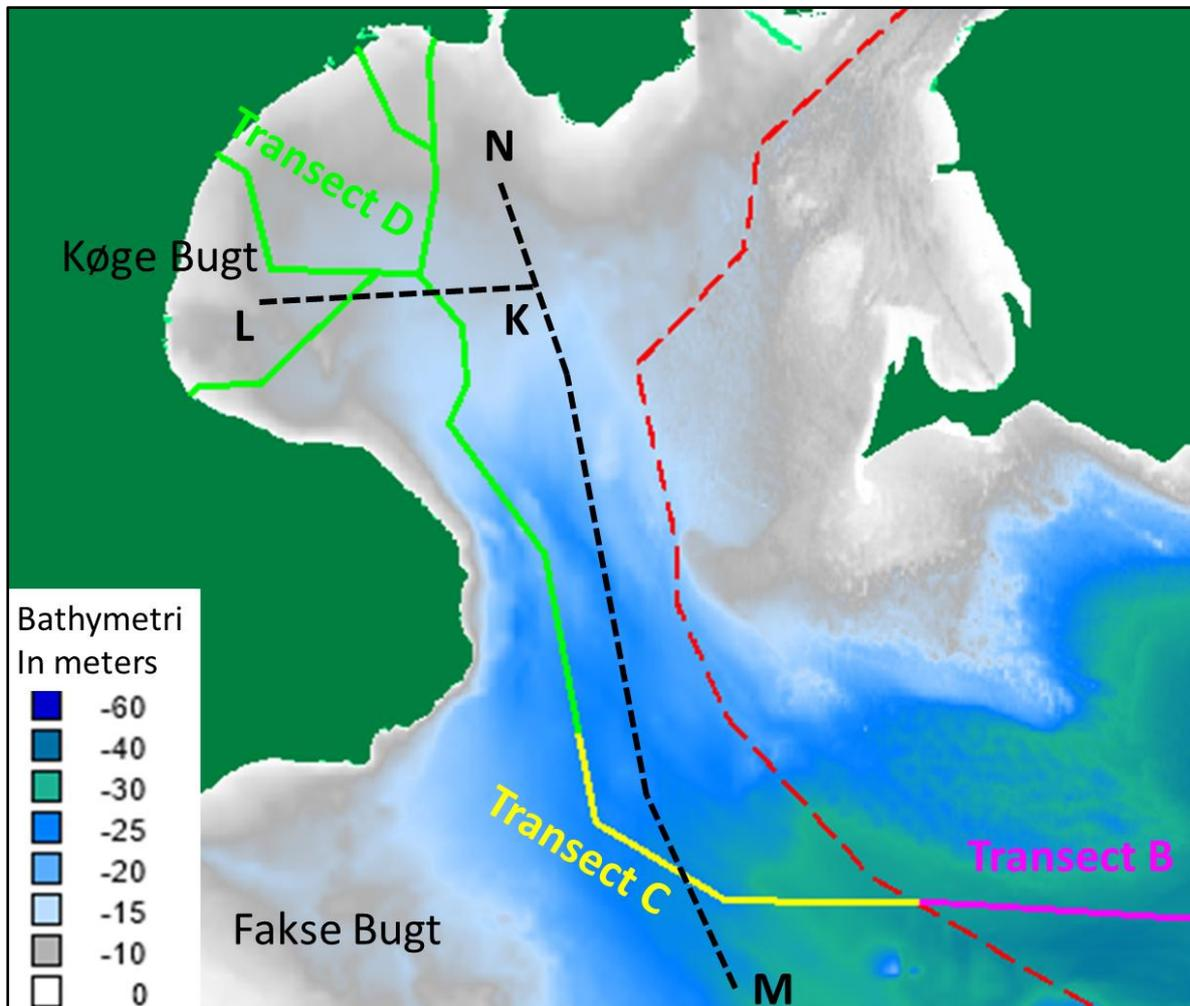
Figure 8.22 Bathymetry in the transect D area. Location of Baltic Pipe profiles sections L–K, and N–M is indicated.
