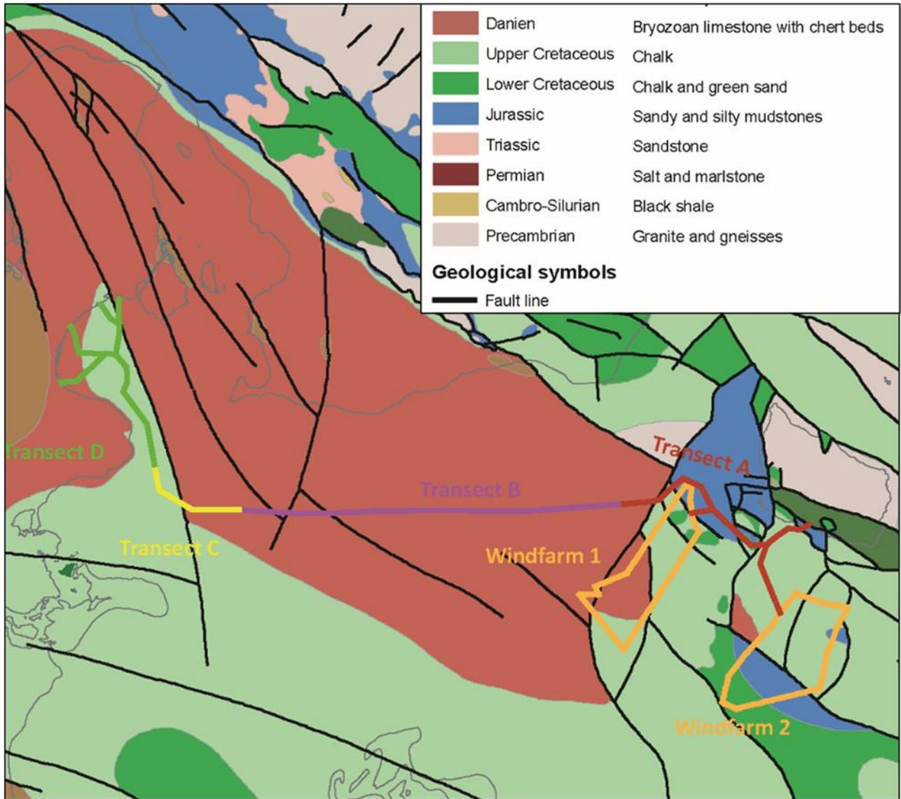
Figure 4.2 Bedrock geology in the cable transect area from Køge Bugt to Bornholm. From Varv (1992). Cable transect A–D is indicated.
