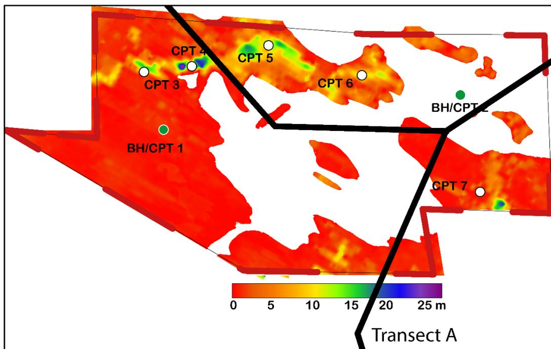
Figure 8.14 Combined thickness of glacial meltwater sand and till. Locations of Transect A, Boreholes and CPT's are indicated.
