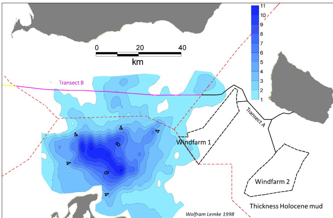
Figure 5.13 Thickness of Holocene mud mapped by Lemke (1998). The locations of Windfarm 1 and 2 (black dashed lines) and cable transects are indicated. The red dashed lines show the EEZ.
