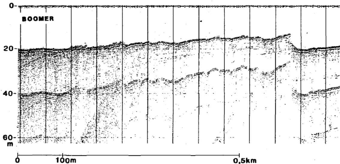
Figure 8.5 Seismic reflection pattern (Boomer) of the Rønne Formation.
