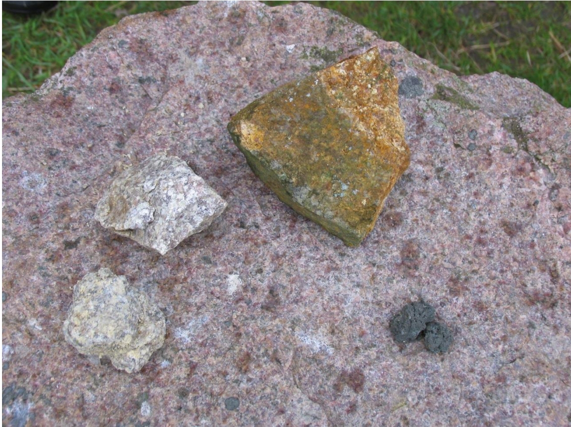
Figure 38. Fine-grained un-weathered Hammer Granite with characteristic red dots in the background. The four smaller fragments on top of the granite represent different levels of weathering: One fragment has yellow-brown coating of iron oxides, two grey and white fragments display different degrees of kaolin weathering. The black fragment of manganese oxide was formed in a fracture. Width of the picture is approximately 50 cm.
