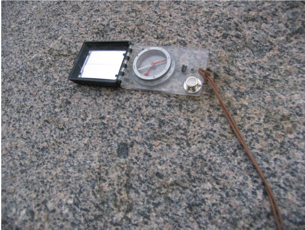
Figure 27. The red and grey, medium to coarse-grained Vang Granite from an unweathered surface in the Vang Quarry.
