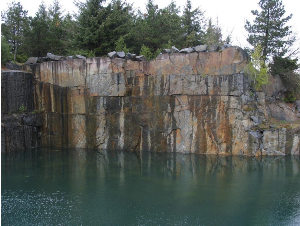
Figure 23. Paradisbakke Migmatite exposed in the Præstebo quarry (exposure height is approx. 12 meters). The distance between horizontal fractures is increasing downwards. Vertical fractures seem to be absent.
