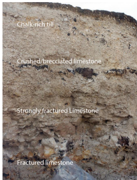
Figure 27. Glacially crushed/brecciated and fractured København Limestone Formation at Limhamn, Sweden (Jakobsen 1994).
