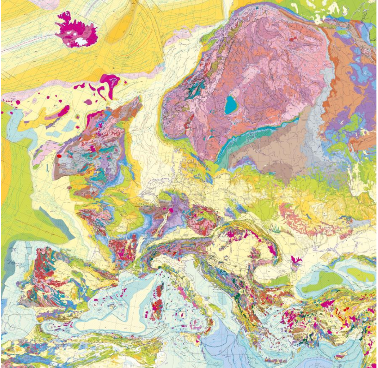
Figure 5. European geological map. The sedimentary basins are in general located in the light-yellow coloured areas (Source: IGME 5000).
