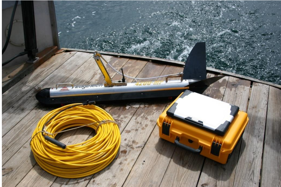
Figur 3-5. EdgeTech 4200 series sidescan sonar.
