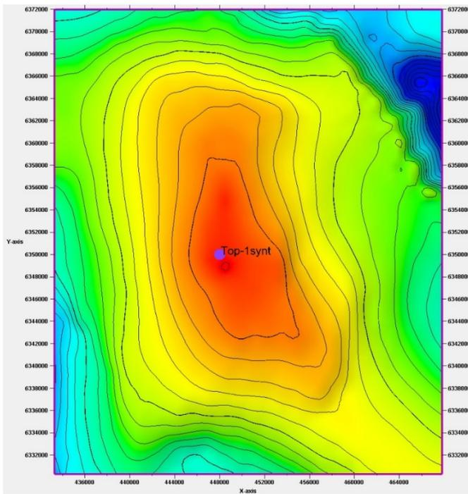
Figure 8. Map of the top Gassum Fm in the model area. The wellhead is placed at UTM 448000, 6350000. For simplicity KB=0. The well penetrates the Top\_Gassum at 908.00 m TVDSS. The structure has its apex at 898 m TVDSS.
