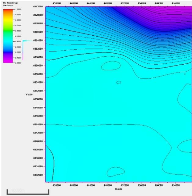
Figure 9. The N/G trendmap for guiding the modelling of the sandstone body distribution. The map reflects the low N/G around the Felicia-1 well in the NE corner, while the main part of the map shows N/G at 41% as in the pseudo-well.
