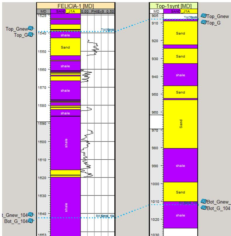
Figure 6. Well sections for Felicia-1 and the constructed pseudo-well Top-1synt for the reservoir section. The porosity log (PHIE) in Felicia-1 is incomplete due to problems with caving in the well bore and therefore only unreliable logging data is available for many intervals.
