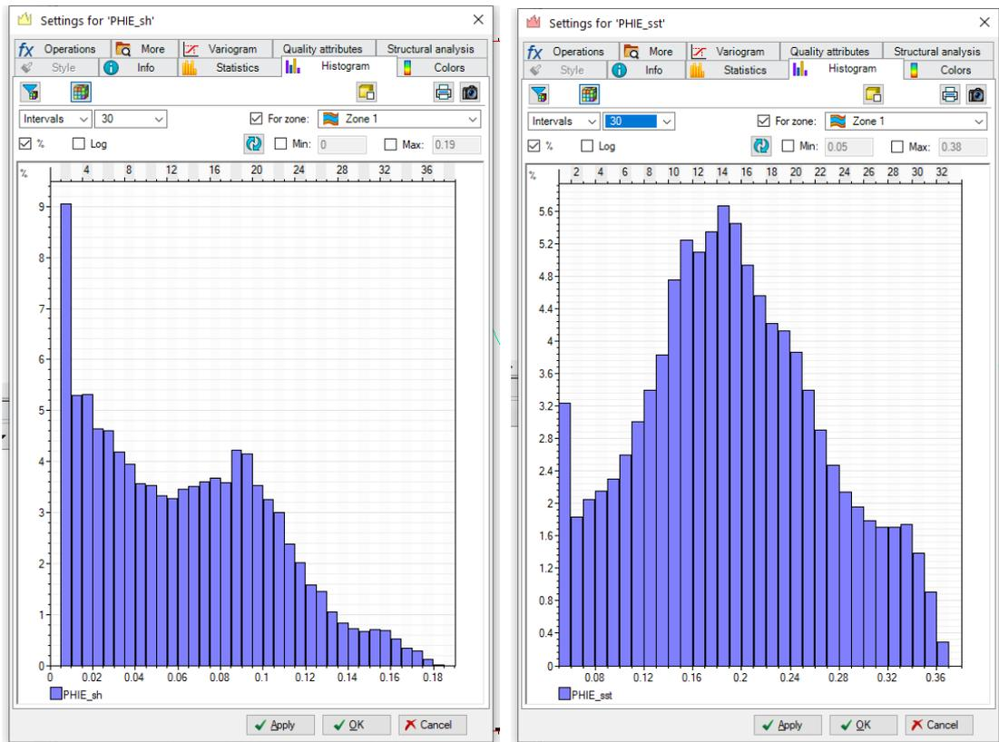
Figure 14. Histograms of simulated porosity illustrating the two populations for the shale and sandstone porosity.
