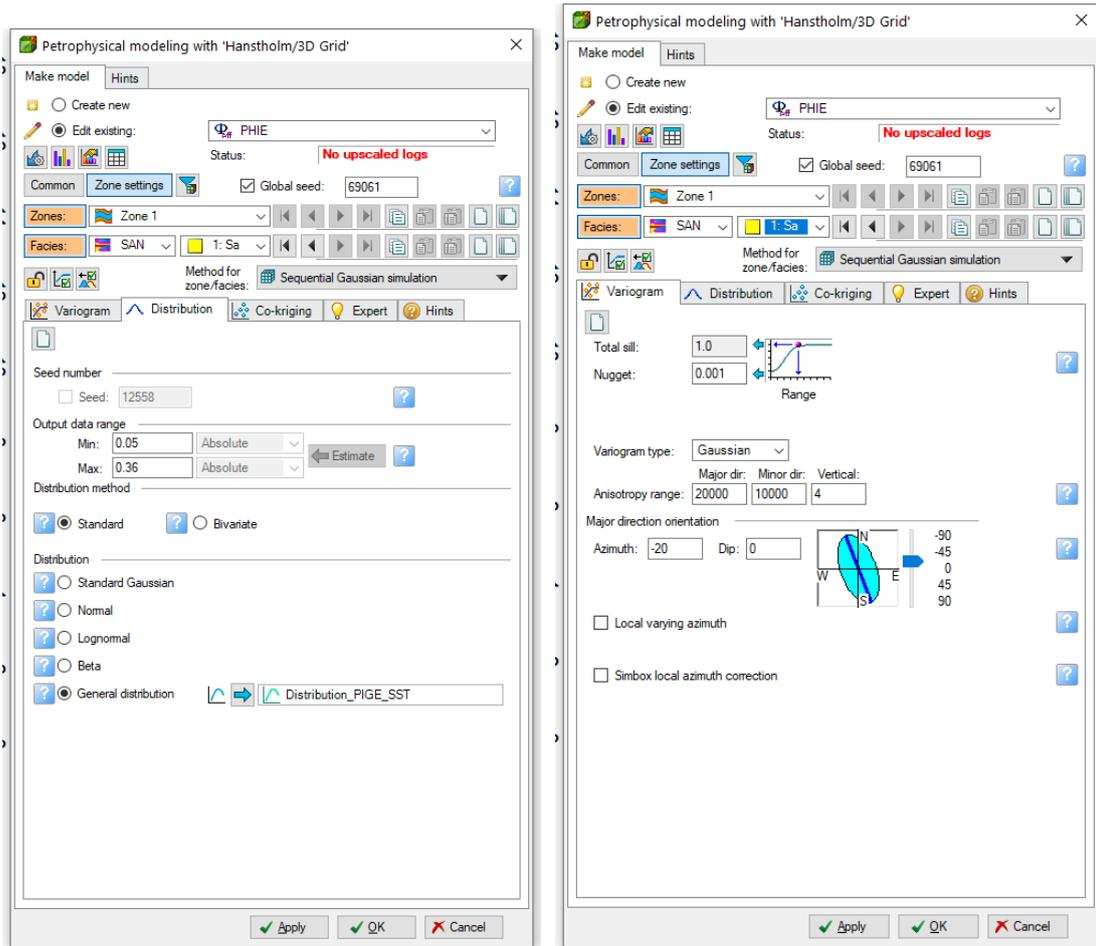
Figure 15. Input sheets for the sand porosity distribution and geometry.
