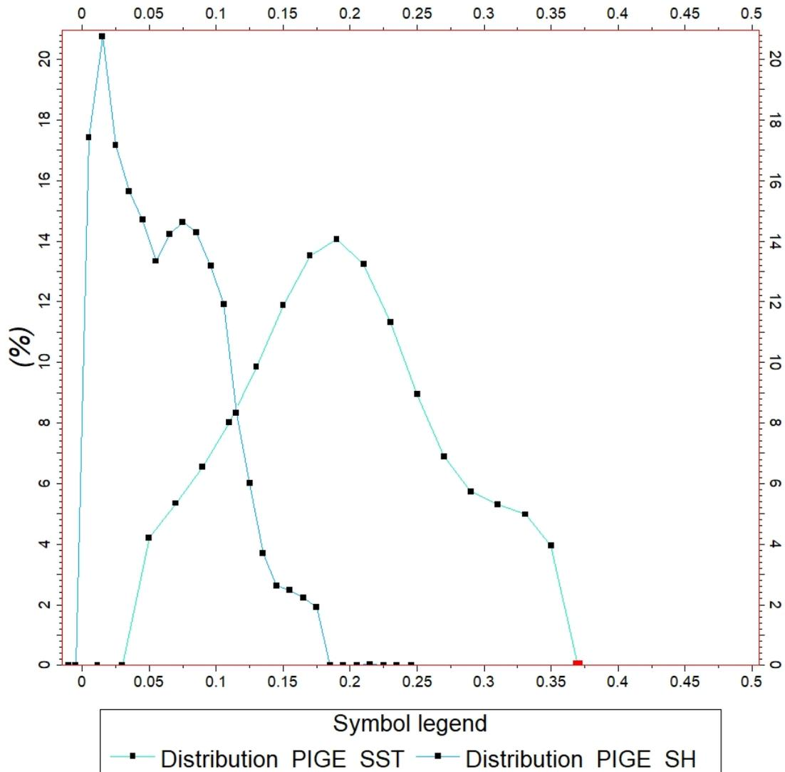
Figure 13. Histograms of porosity target distributions for shale and sandstones.
