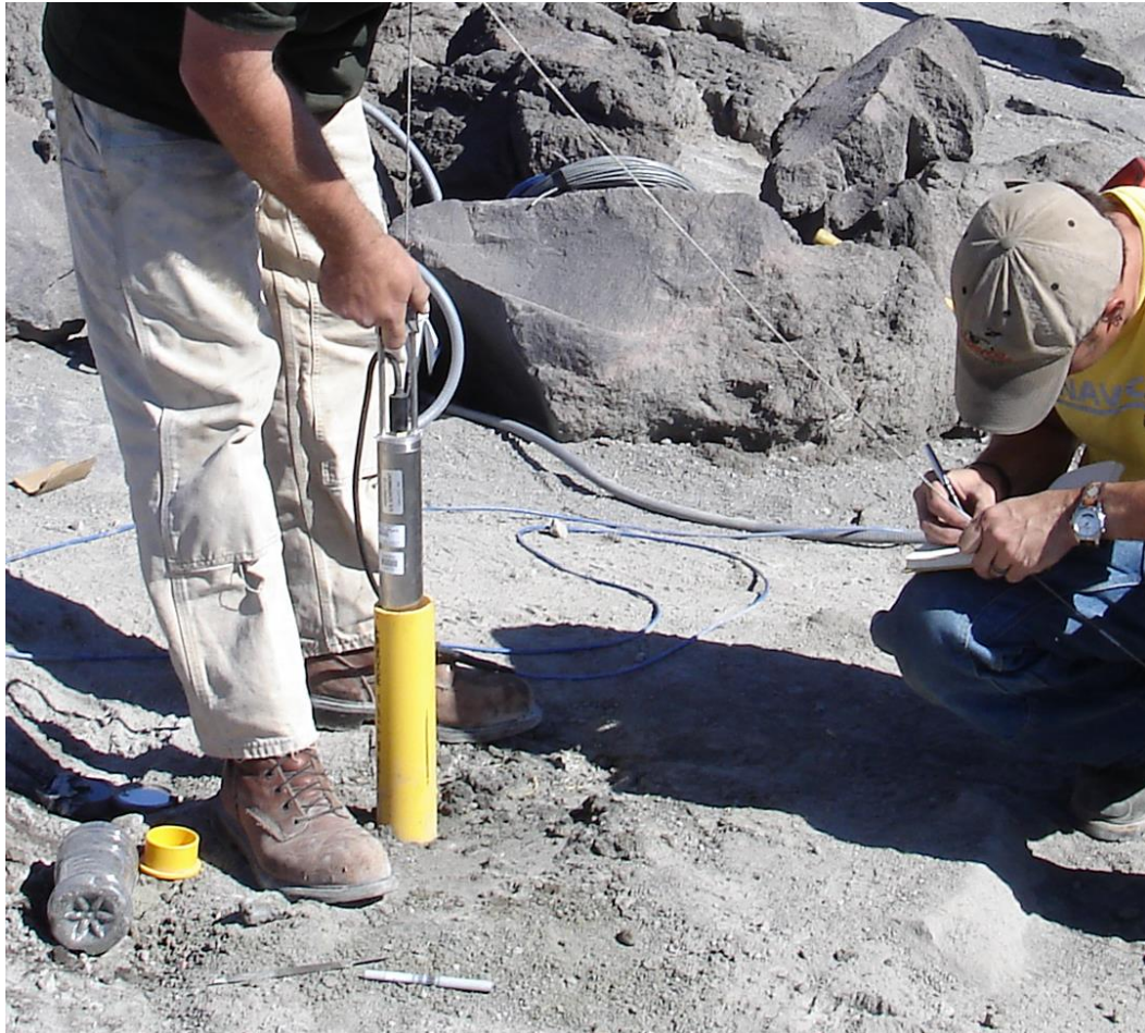
Fig. 3: Installation of tiltmeter in a shallow bore hole. Photo: UNAVCO.
