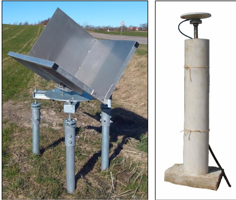
Fig. 2: Left: Corner reflector optimised for Sentinel-1 ascending and descending acquisitions. The reflector is 1 m wide and mounted in an agricultural field on three screw pegs inserted 1,5 m into the ground, Photo: Marie Keiding, GEUS. Right: GNSS station mounted on concrete pillar for long-term or permanent monitoring. Photo: UNAVCO.
