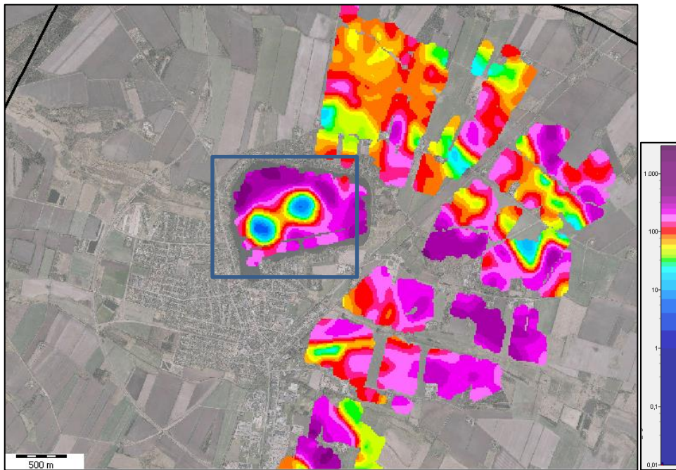
Figure 3.6 2D resistivity grid for tTEM at elevation +30 m. The FloaTEM data on the lake resolves two areas of late-postglacial gyttja deposits with thicknesses up to 20 m (blue/green colours).
