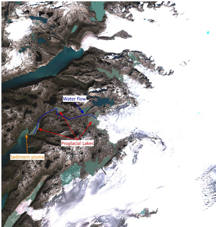
Figure 27. Example of water flow, a sediment plume, and proglacial lakes in a catchment. As water flows through the proglacial lakes, these act as natural sediment traps filtering away sediments. Once the water reaches the fjord the outflow of water containing the remaining sediment will appear as a plume in the surface layers of the fjord water. The base-map is a summer 2018 optical Sentinel-2 satellite image.
