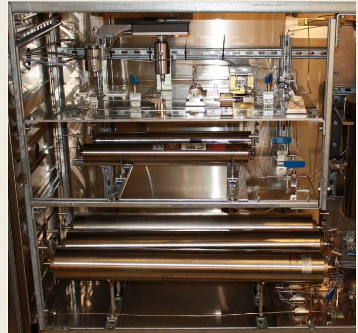
Full Core Rig for samples with diameter up to 12.3 cm
