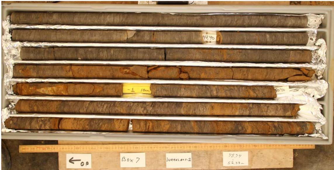
Fig. 15. Core photo from drill site. Box 7: 45.74 – 52.33m
