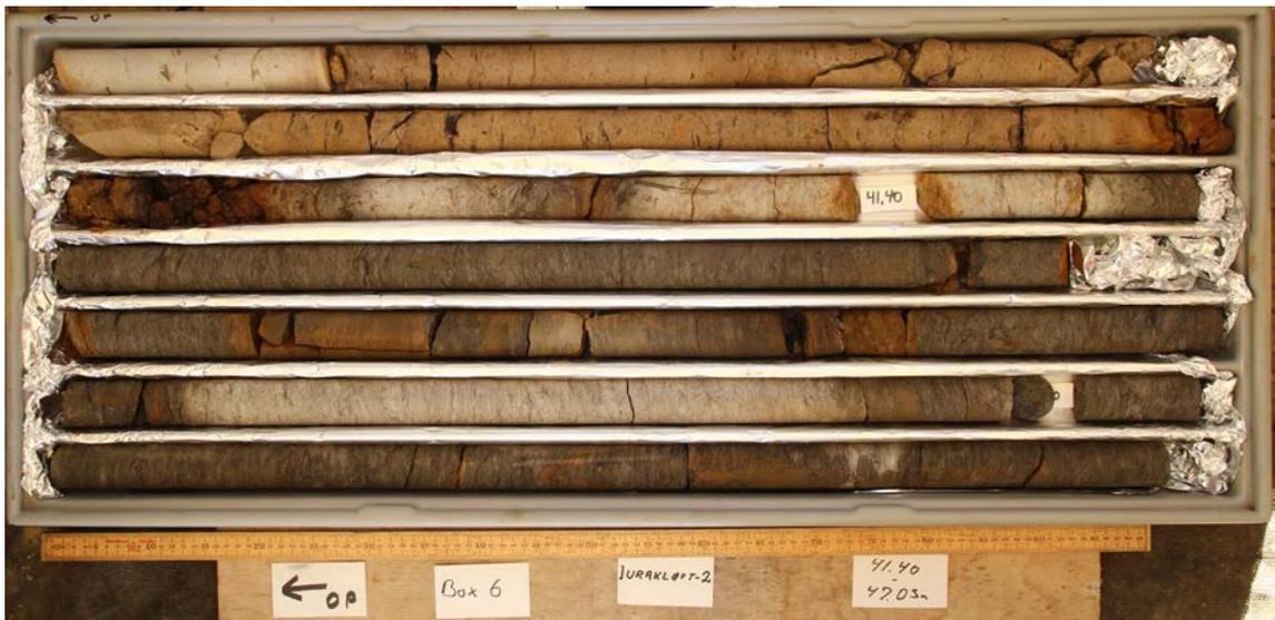
Fig. 14. Core photo from drill site. Box 6: 41.40 – 47.03m
