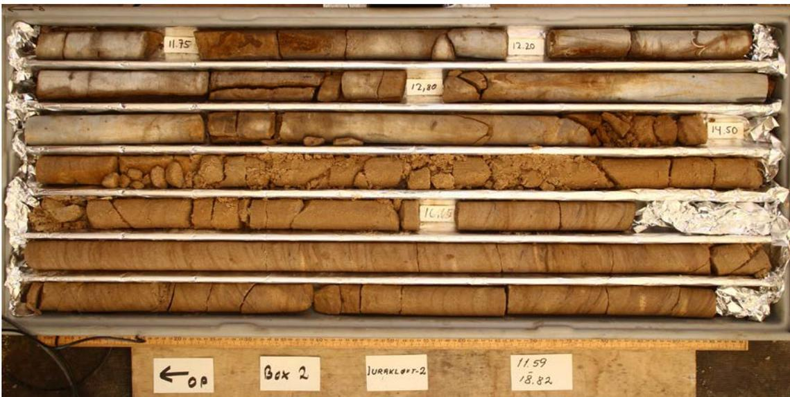
Fig. 10. Core photo from drill site. Box 2: 11.59 – 18.82m
