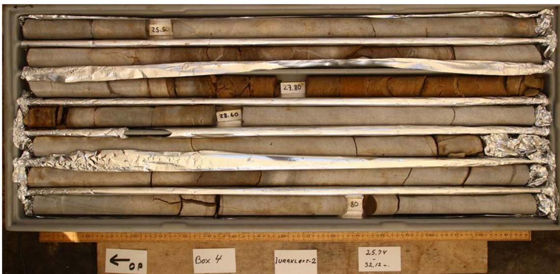
Fig. 12. Core photo from drill site. Box 4: 25.94 – 32.12m
