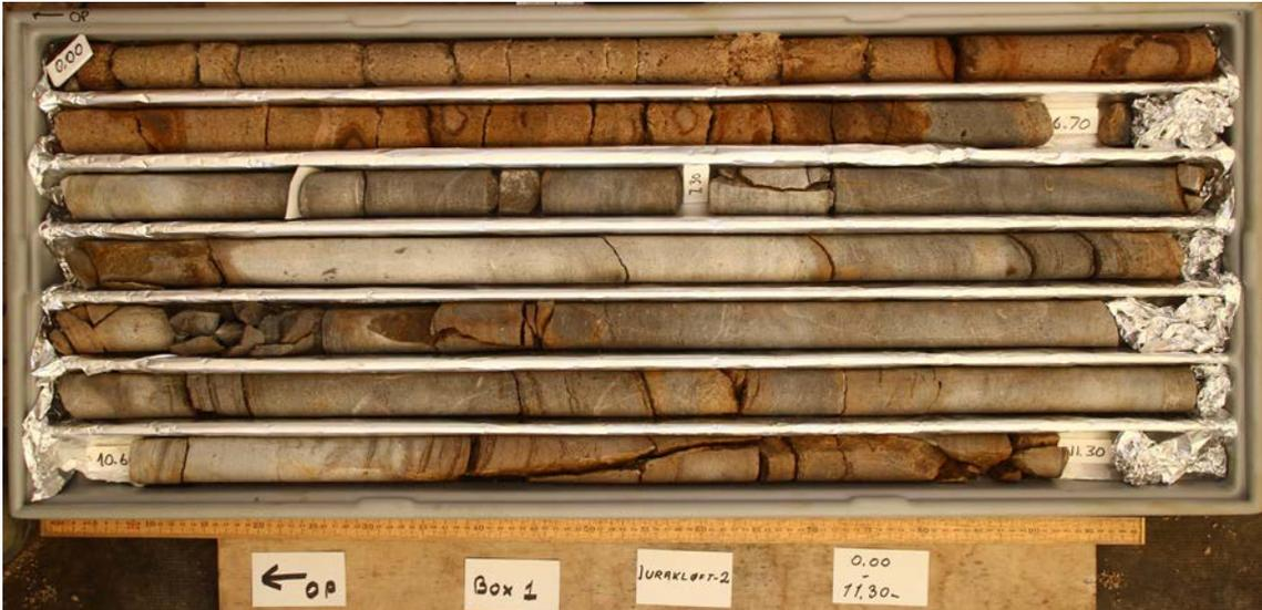
Fig. 9. Core photo from drill site. Box 1: 0 - 11.30m
