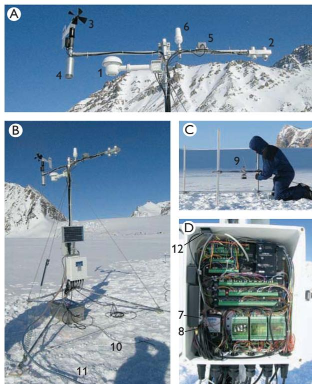
Fig. 2. Standard sensor suite of the automatic weather station on Arcturus Gletscher at the Malmbjerg molybdenum prospect. **A:** The main instrument boom. **B:** The tripod and the sites of the thermistor string and pressure-transducer assembly drilled into the ice. **C:** The sonic ranger-stake frame drilled into the ice. **D:** The inside of the data logger enclosure. The numbers refer to the list in Table 1.
