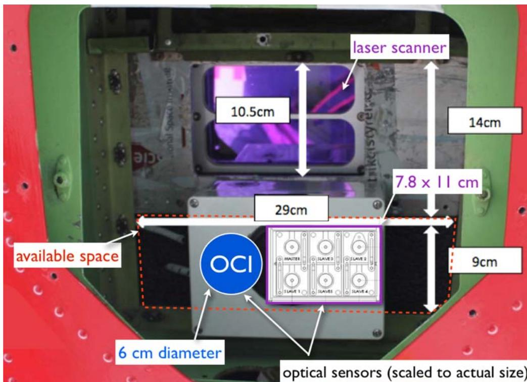
**Figure 8.** Twin Otter belly port, photographed from below, showing the locations of OCI hyperspectral and MCA multispectral cameras complimenting the laser altimetry measurements.
