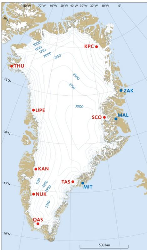
**Figure 1.** Location and identification codes of PROMICE automatic weather stations. The ZAK and MAL stations are GEUS stations from other projects. The KAN stations are mostly financed by the Greenland Analogue Project (GAP), a PROMICE collaborator. Dotted lines are elevation contours in m above sea level.
