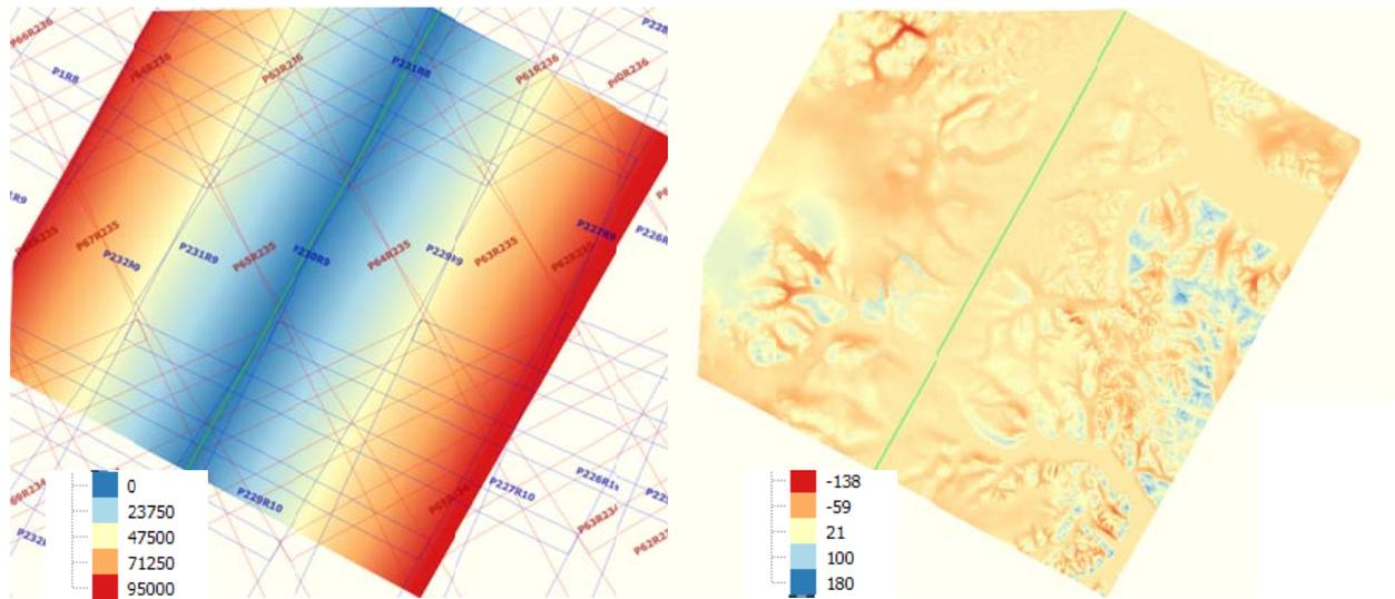
**Figure 13.** *a: across-track distance in metres from the satellite ground track (marked by the green line); b: calculated total horizontal error in metres in the across-track direction for WRS2 path 230, row 9 due to the inaccurate DEM. The scene has sides of ca. 190 km.*
