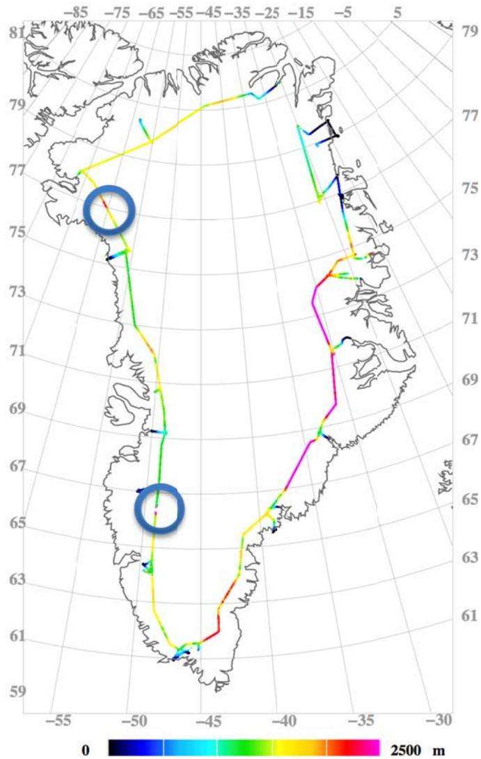
**Figure 7.** Ice sheet elevations derived from the PROMICE 2015 airborne campaign. Circles indicate areas where outliers caused by clouds are evident.
