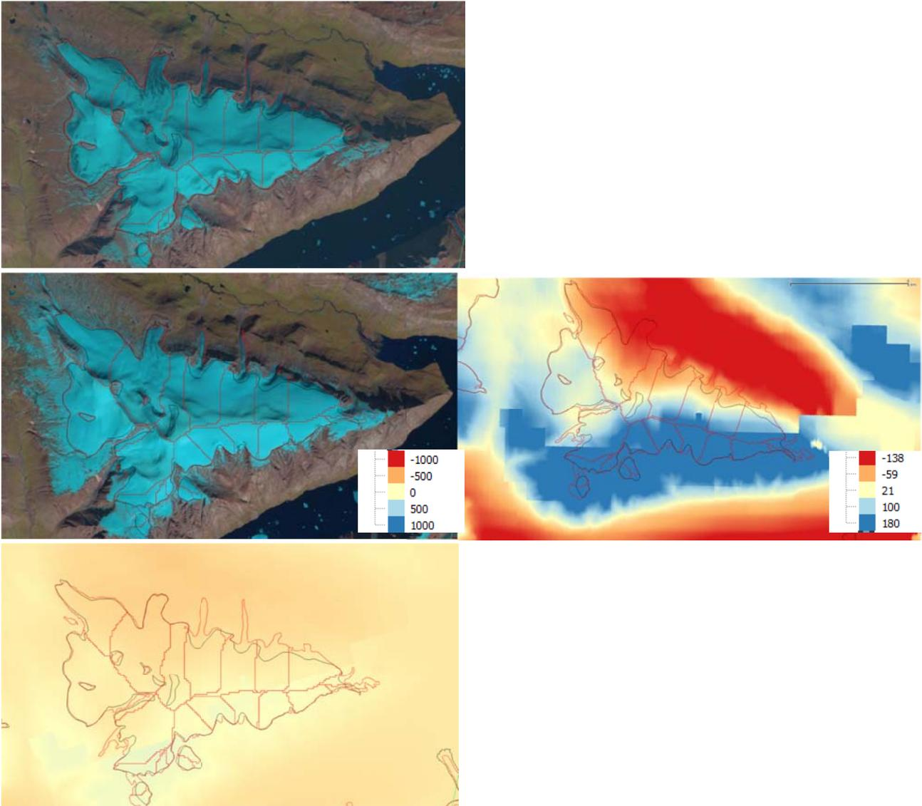
**Figure 14.** Enlarged example of large DEM error introducing co-registration errors between two scenes from path 230, row 9, year 2015, DOY 183; bottom image: path 231, row 9 year 2015, DOY 174.
