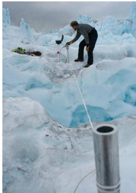
Installation of (left) crevasse water monitor float and (right) crevasse strain gauge at Store Gletscher.
