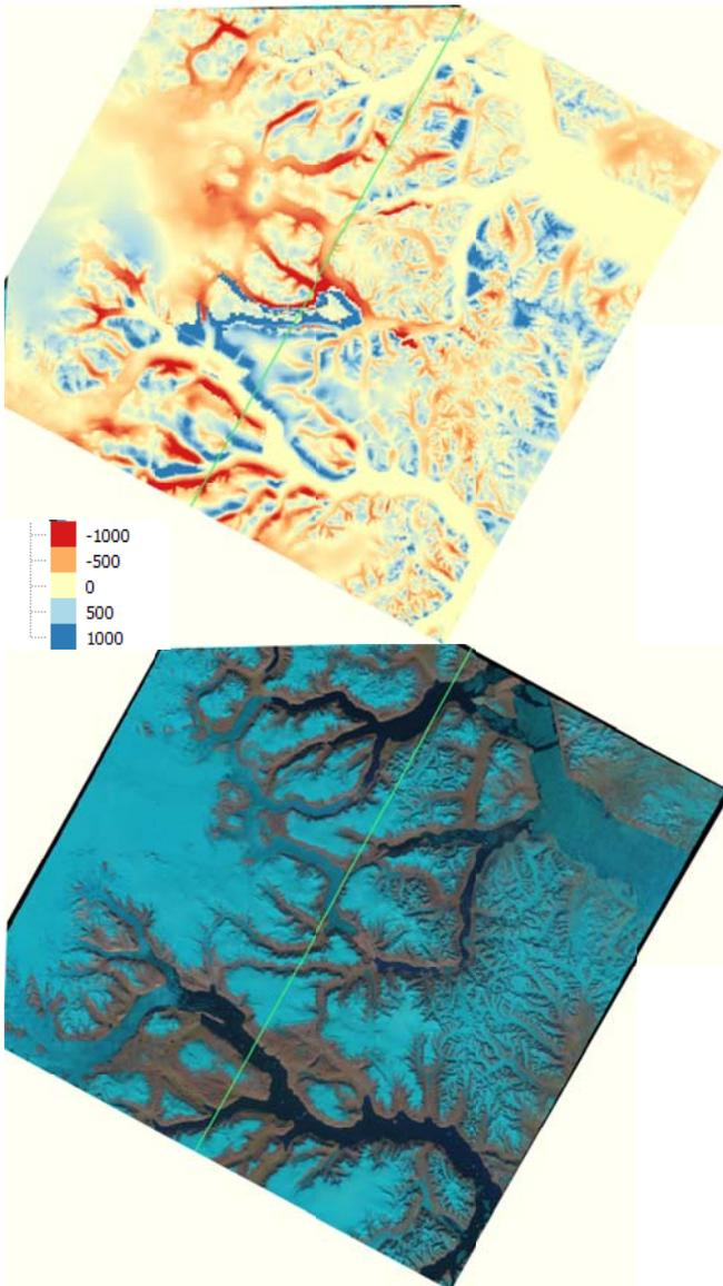
**Figure 12.** *a: elevation difference between GSL DEM and GIMP DEM; b: Landsat 8 false color composite overview of the region in central east Greenland used as an example throughout this section. The scene has sides of ca. 190 km.*
