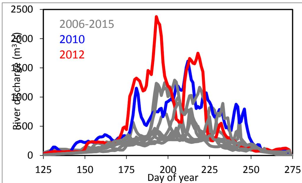
**Figure 20.** Preliminary results for the recalculated daily-mean discharge estimates from Watson River.
