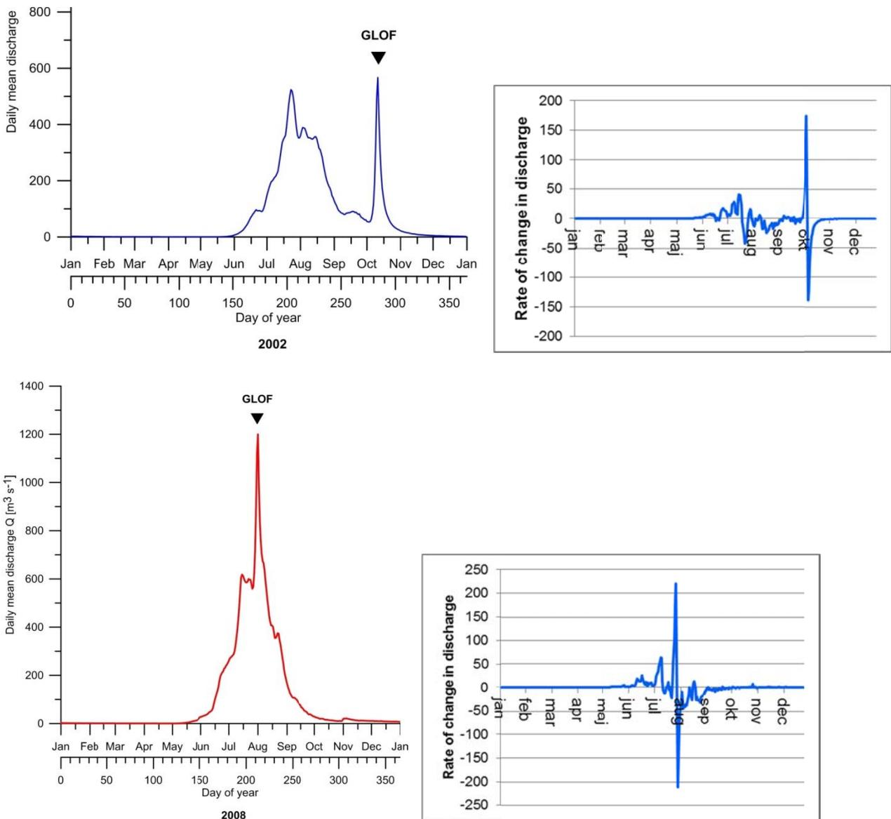
**Figure 17.** Annual discharge curves showing sudden peaks related to glacial lake outburst floods. Note how the rate curve (inserted graphs) has a clear signature, revealing the GLOF even when it occurs in the middle of the peak discharge of the main catchment.
