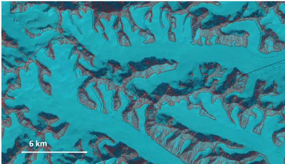
**Figure 10.** Landsat 8 L1T details over the upper basins of Schuchert Glacier and Storgletscher (Stauning Alps), showing E-W error at places exceeding 200 m. Top image: path 227, row 9, year 2015, DOY 178; bottom image: path 230, row 9 year 2015, DOY 185. Red and black lines respectively from the glacier inventory of Rastner et al, 2012 and the PROMICE glacier map of Citterio & Ahlstrøm, 2013.
