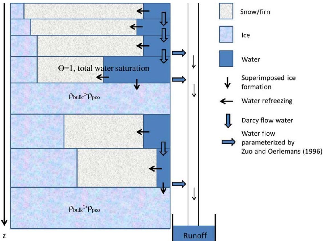
**Figure 21.** Schematics of idealized water percolation and retention in HIRHAM5 subsurface scheme.
