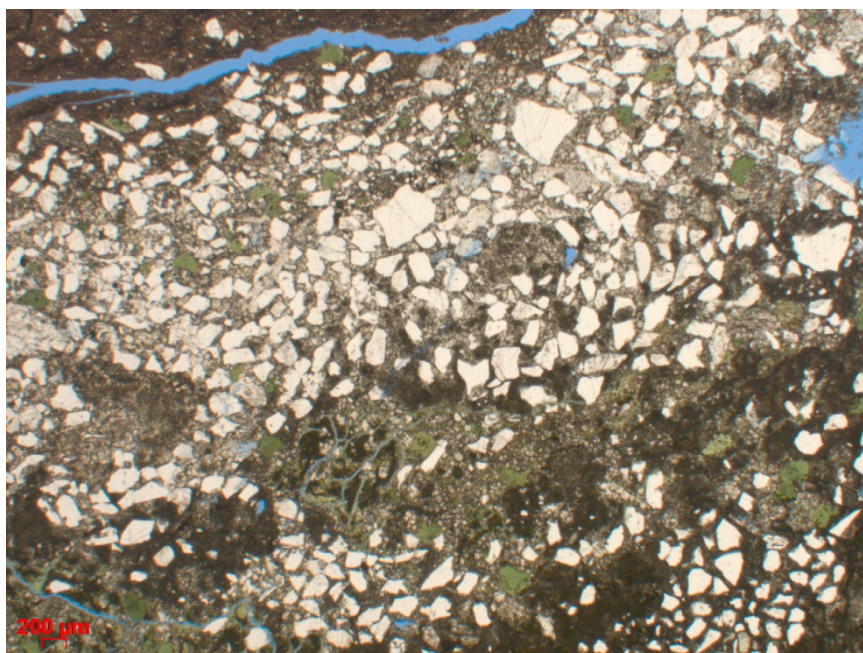
Figure 5.17. 133.30 m. Detrital grains, dark brown carbonate clasts and greenish glauconitic pellets in sideritic and ankeritic cement.
