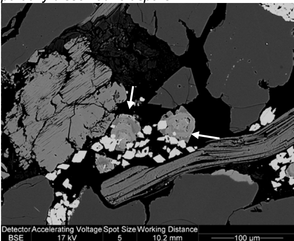
Whitish rhombs of siderite scattered and some engulfed by patchy ankerite (arrows). Note incipient quartz overgrowths, kaolinite booklets and partially dissolved K-feldspar (BSE image).
