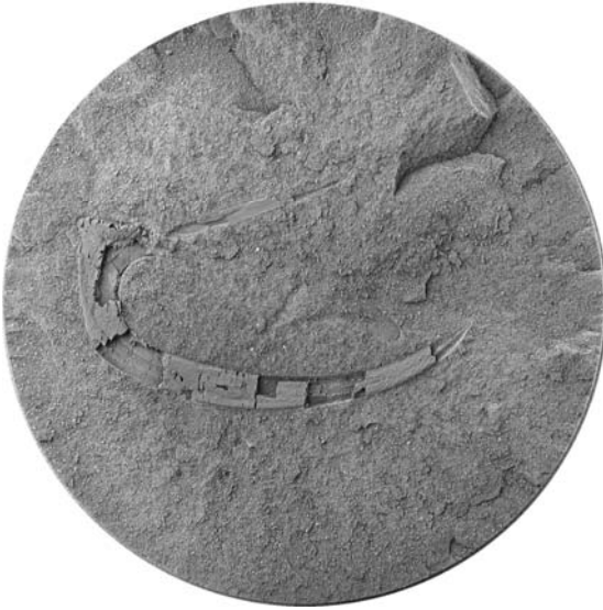
Figure 3.2.3: Onychites , hook from belemnite, from depth 34.01 m Diameter of core is 56 mm.
