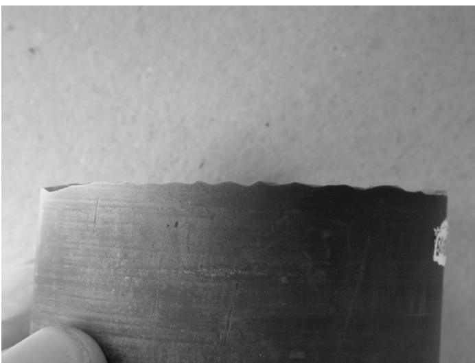
Figure 3.2.5: Core piece viewed from side showing characteristic crenulations of bedding plane formed by ammonite ribbing. Diameter of core is 56 mm.
