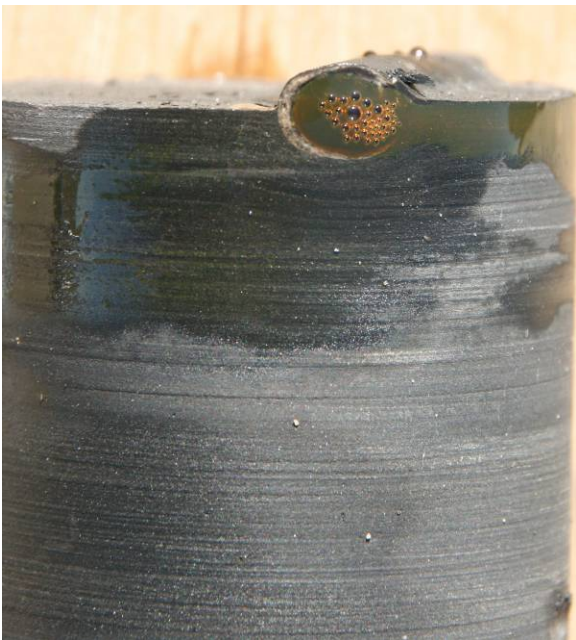
Fig. 7.1.2. Bitumen found in a fracture within an igneous intrusion at 55.4 m, and oil observed within a belemnite at 105.25 m. See Section 7.2.
