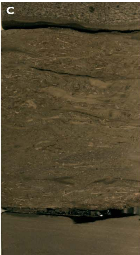
Fig 4.4. Core photographs of the Upper Jurassic Katedralen Member (Hareelv Formation); core section height: 10 cm. A–B) Mudstone conglomerates 71.2–71.4 m. C) Muddy shell bed overlying a coalified wood fragment, 83.5 m. D) Bentonite bed, 82.6 m.
