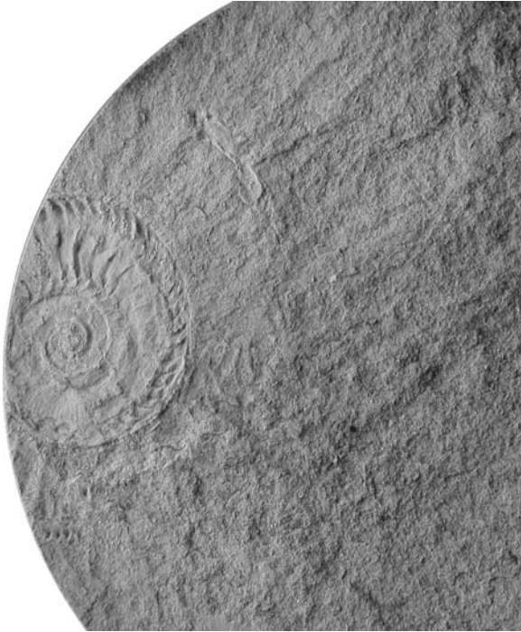
Figure 3.2.25: Cardioceras ( Cawtoniceras ) aff. blakei Spath or cawtonense (Blake & Huddleston) (GGU 511101-432) at level 211.30m indicates faunal horizon M8 and the C. tenuiserratum Zone. Diameter of core is 56 mm.
