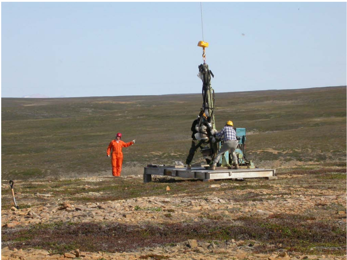
Fig. 2.1 Assembling the drill rig.
