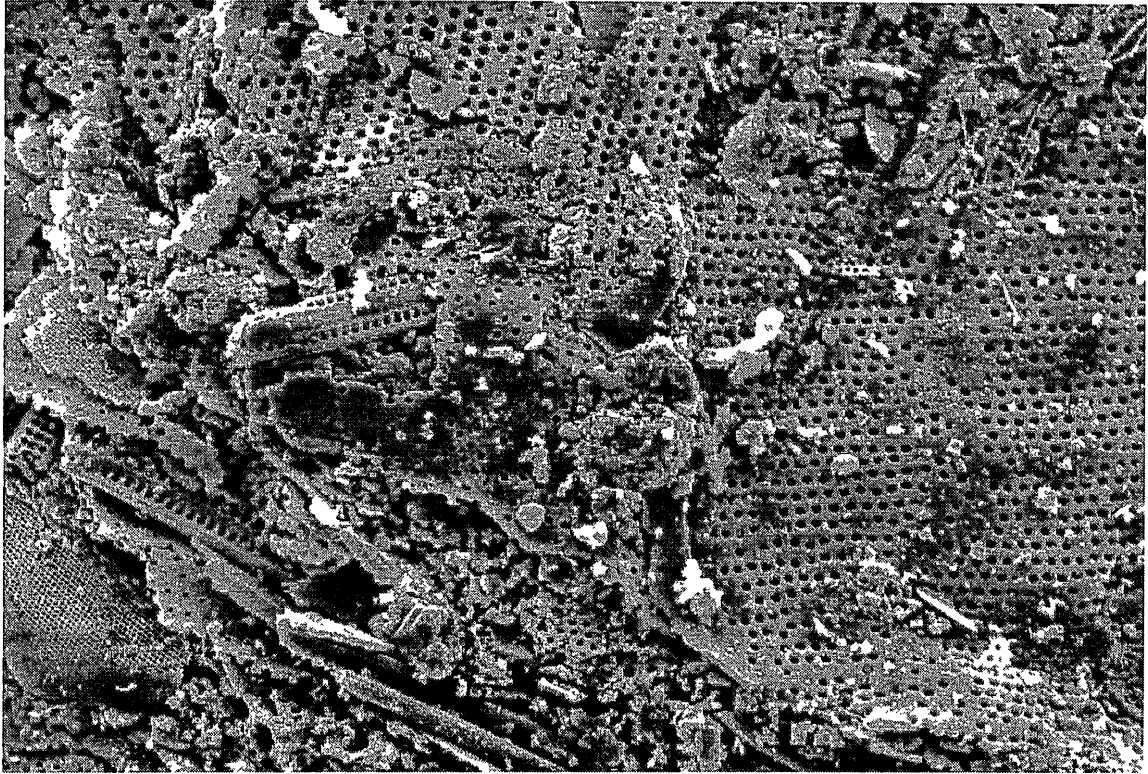
Figure 9. SEM microphoto showing the surface of large diatoms from the Zakynthos sample ( Actinocyclus sp.?). Note that calcite had not been removed from this sample prior to this SEM investigation. Photo frame c. 100 \mu m wide.
