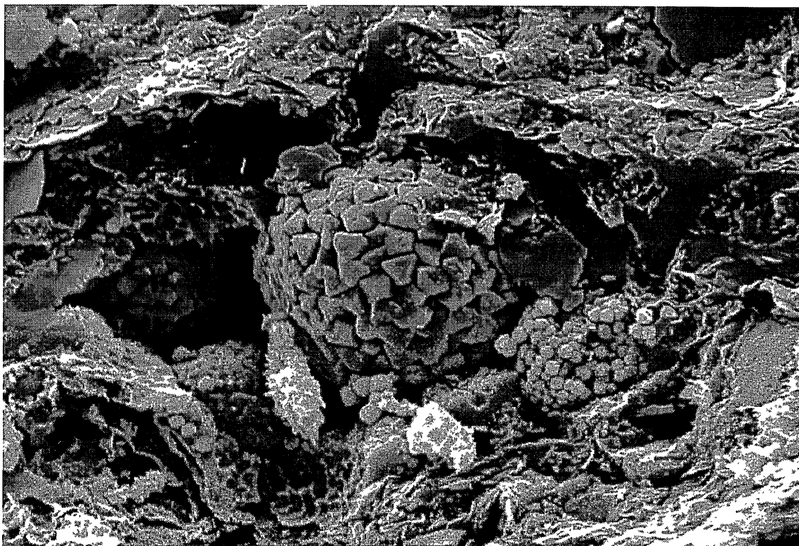
Figure 4. SEM microphoto of framboidal pyrite in chertified layer. Note that the framboid in the center contain tetrahedral pyrite crystal while the framboid to the right only contains semicrystalline pyrite. Size of big framboid is 10 my.
