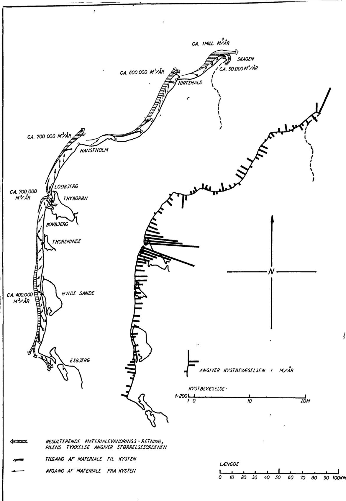
Figure 16. The left side: net sediment transport and direction at the westcoast of Jutland. Arrows indicate erosion of or deposition at the coast. The right side: Coastal displacement measured in mm/year. The database is averaged values from the century 1868-1968. From Nielsen & Nielsen, 1982.
