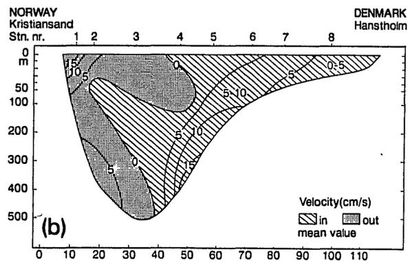
Figure 5. (a) Surface currents in the Skagerrak (Swansson, 1975). (b) Cross-section of the Skagerrak showing in- and outflow patterns (Rhode, 1987). From Kuijpers, 1993.
