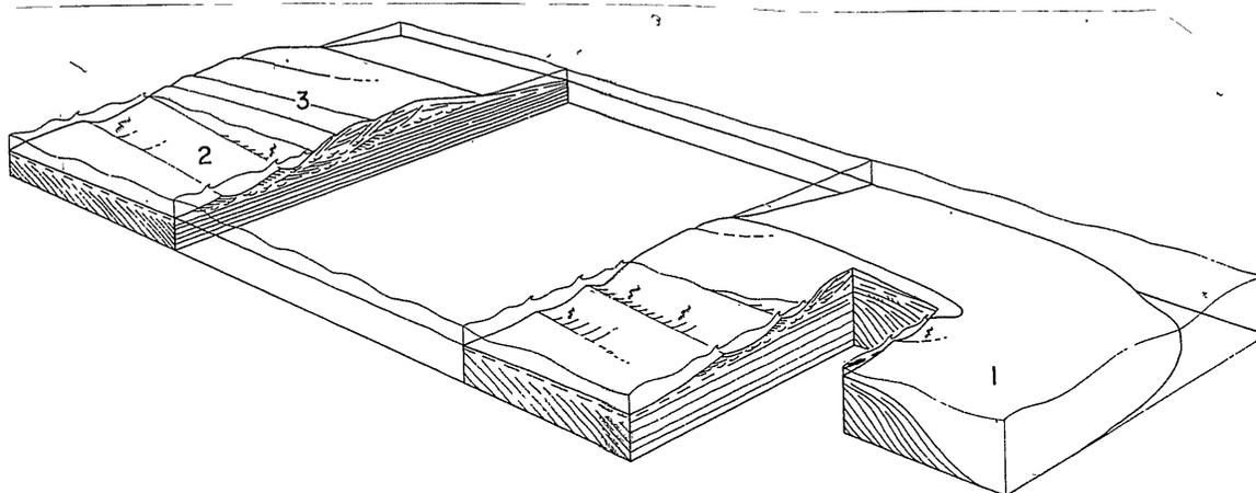
Figure 19. Dynamic three-dimensional morphological-sedimentological model for coarse-grained spit systems prograding into deep water: 1. Spit platform; 2. Oblique bar-trough system; 3. Spit, beach. From Nielsen et al., 1988.
