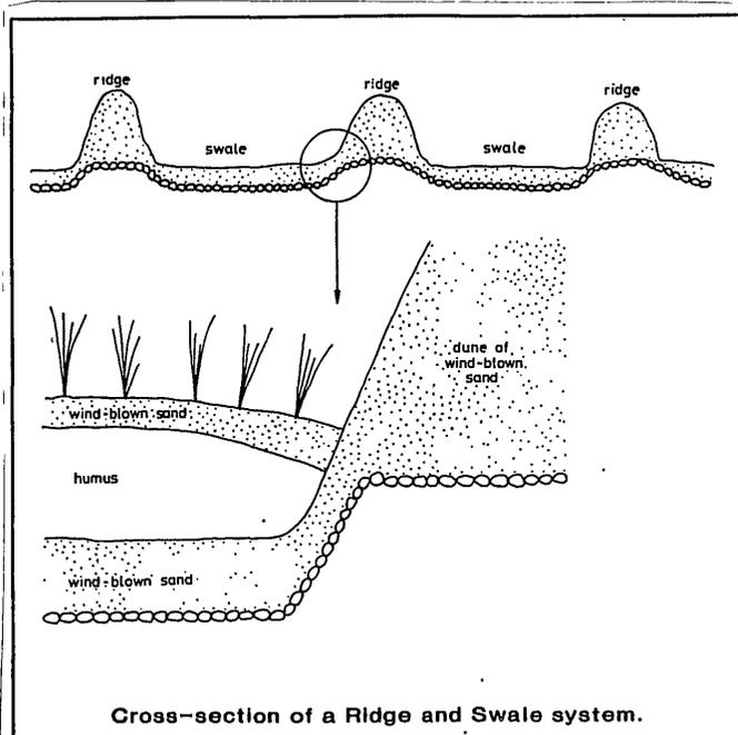
Figure 7. Cross-section through part of a 'ridge and swale system' typical of an area of coastal advance (like Skagen Nordstrand today). The system develops perpendicular to the coastline. The distances between the ridges may vary according to the frequency of storms i.e. increasing numbers of storms, the greater number and the higher concentration of beach ridges. From Hauerbach, 1992.
