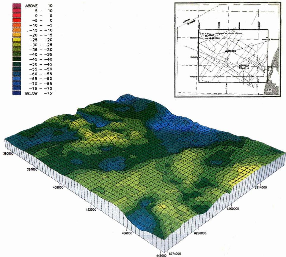
Figure 23. 3-D view glacial contour map showing the modified topography of the glacial surface in the Jutland Bank area. View from the southeast to the Northwest across the study area. Contour interval, 5 metres. The numbers on the sides indicate UTM eastings and northings (UTM-zone 32). From Leth, 1996.
