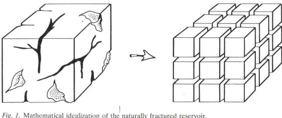
Fig. 1. Mathematical idealization of the naturally fractured reservoir.
