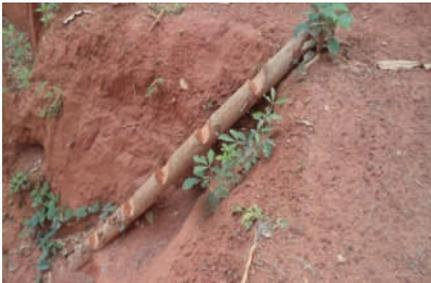
FIGURE 2.24 | EXEMPLE DE TROU AYANT PROVOQUÉ LA CHUTE D'UN MINEUR ARTISAN À CAUSE DE LA NON-CONFORMITÉ DE L'ÉCHELLE (CAPAM).
