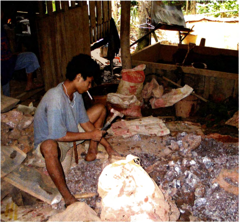
Fig. 3-11. Crushing gold ore with hammer (Philippines).
