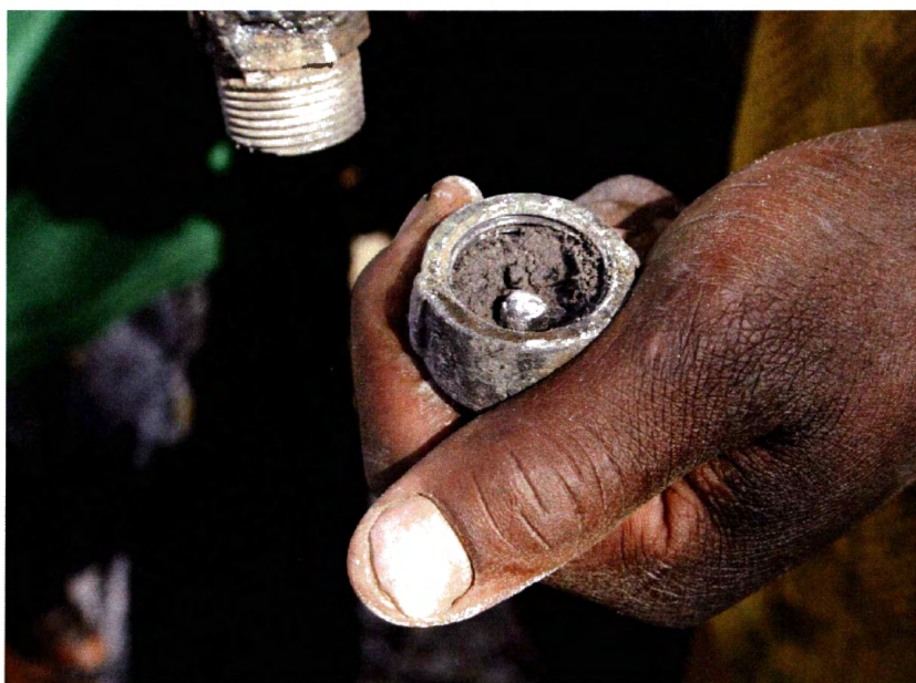
Fig. 5-13. Amalgam (mercury – gold mixture) ready for burning in the retort
