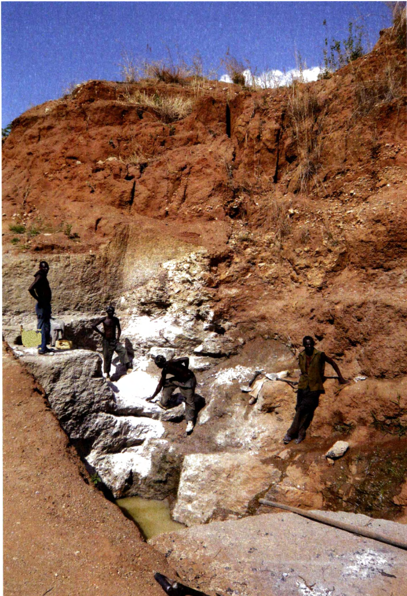
Fig. 3-5 Aquamarine prospect in Lundazi. An excavator has dug through the overburden to the hard rock with aquamarine. Mining of aquamarine is done by hammer and chisel.
