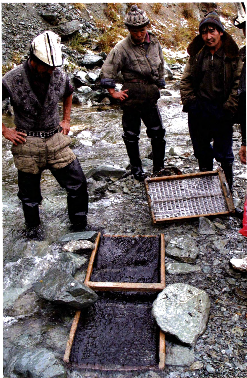
Fig. 3-14. Sluicing for gold in a stream in Kyrgyz Republic.
