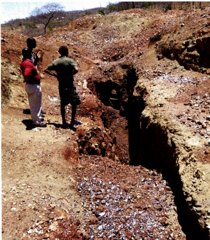
Fig. 3-4. Amethyst vein. The overburden seen in the background has been removed by bulldozer. Mapatizy area in Kalomo.
