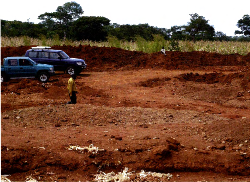
Fig. 3-7. A bulldozer has removed the overburden covering a topaz deposit. The overburden is placed around the topaz deposit e.g. behind the cars. If the small-scale miners have sufficient funding they should be able to level the ground again with a bulldozer when they have exhausted the deposit.
