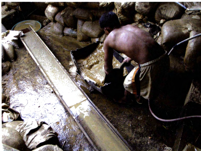
Fig. 3-16. Rinsing sluice carpet for gold in the Philippines.
