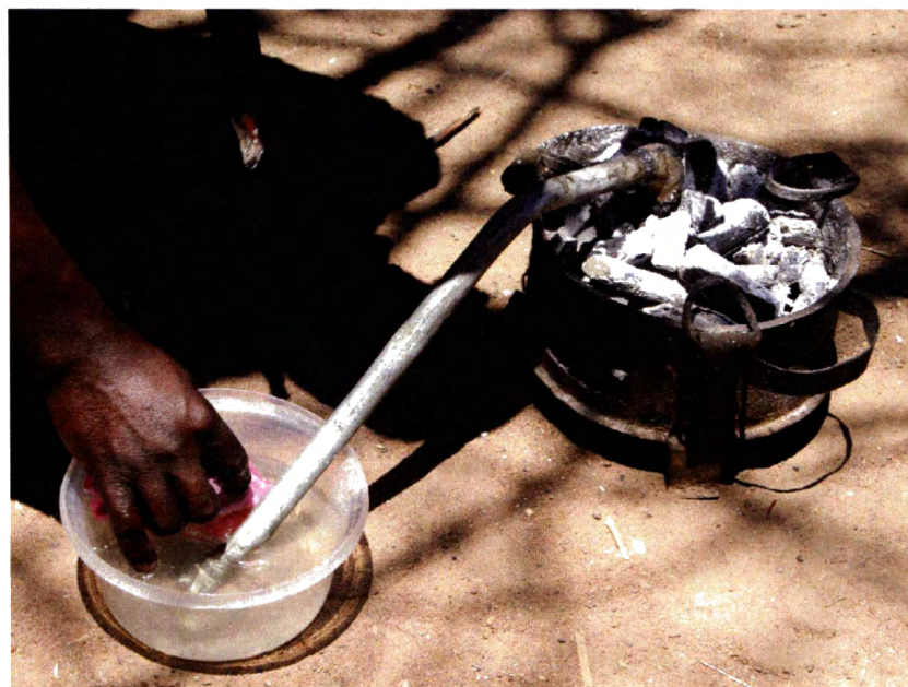
Fig. 5-15. Heating the retort over a charcoal burner.
