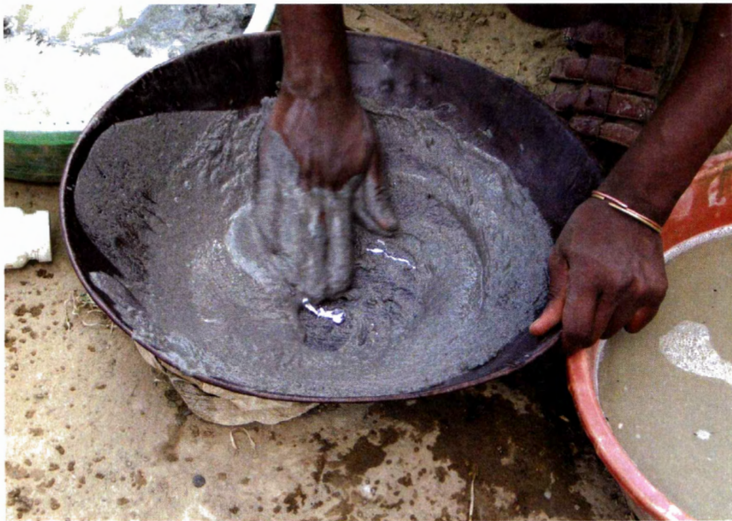
Fig. 3-18. Mercury added to mineral concentrate for gold extraction in Tanzania.
