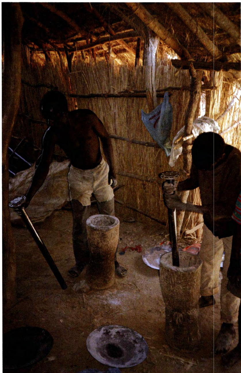
Fig. 3-12. Grinding gold ore by car axles in tree stems in Tanzania.
