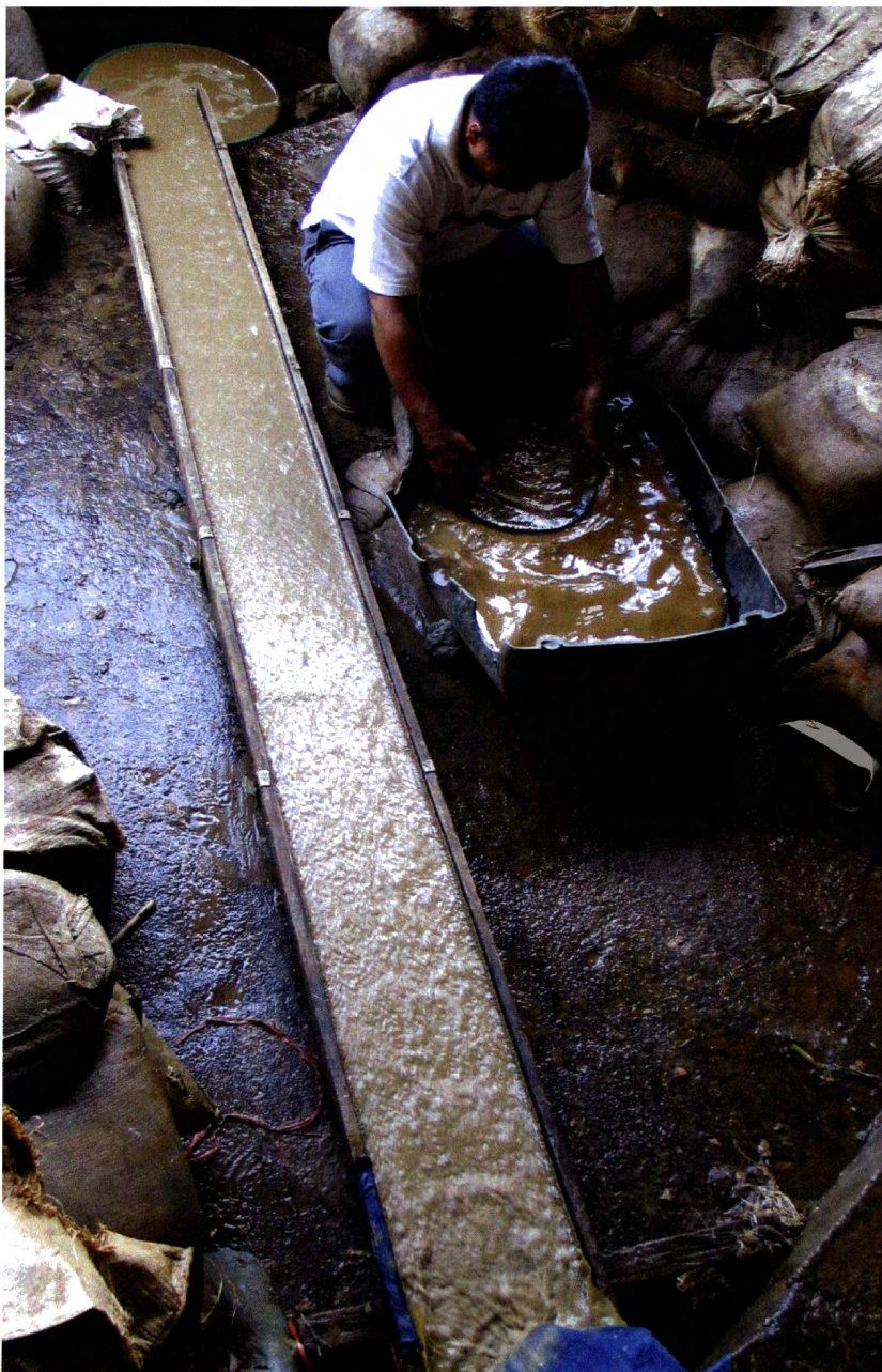
Fig. 3-15. Sluicing with carpet in Philippines.
