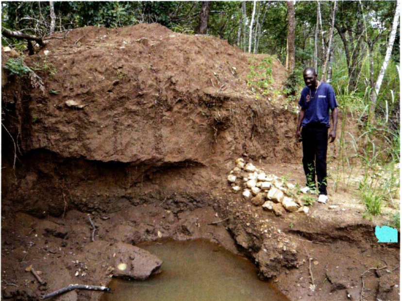
Fig. 3-8. Alluvial (placer) gold deposit (the c. 30 cm thick pebbly layer). The overburden is removed and the gold-bearing layer is mined with shovels. In this case the overburden was not dumped in an environmentally safe place, but was thrown directly into the stream and washed away, thereby clogging up the drainage system. The gravel, sand and silt in the gold ore have likewise been dumped into the stream.
