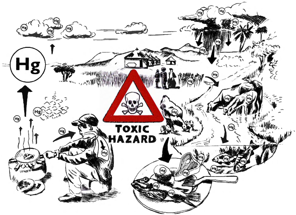
Fig. 5-8. Paths of mercury in the environment and the food chain. Hg is the chemical symbol for mercury. The “story” starts in the lower left corner and goes on clockwise. A small-scale miner burns amalgam and thereby releases metallic mercury. He inhales some of the mercury. The rest of the mercury falls down on the soil with the rain. Then the metallic mercury is converted to methylated mercury and enters the food chain through the drainage system and ends up in cows, hens and fish. When eating them the population is poisoned by methylated mercury.
