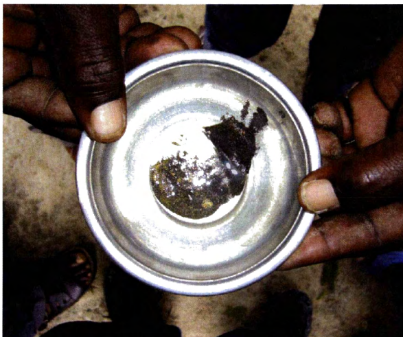
Fig. 5-12. Small pan for producing a gold concentrate.
