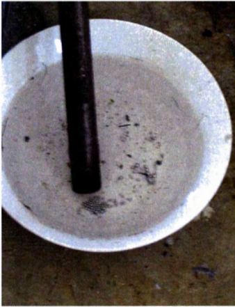
Fig. 5-16. Mercury condenses in a bowl of water and can be used again and again.
