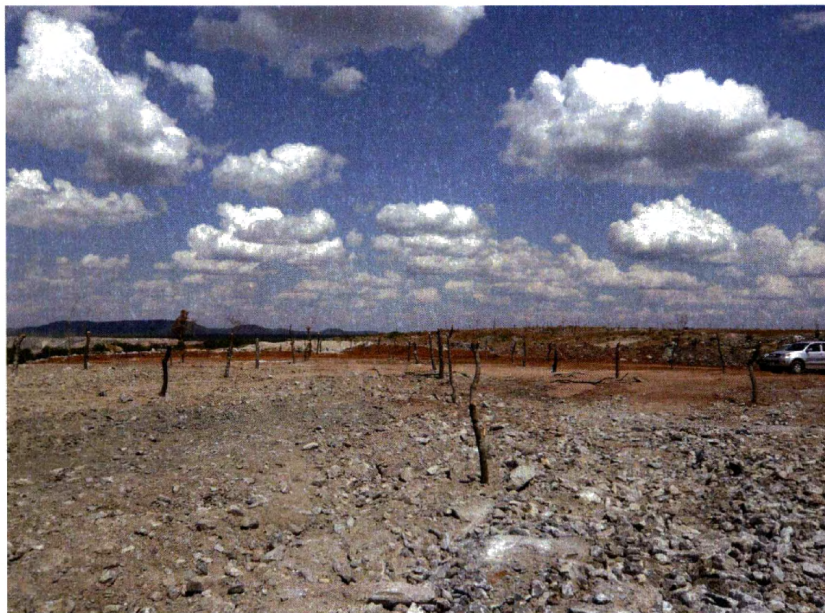
Fig. 5-6 shows an emerald mine in the Lufwanyama Emerald Area where a large number of trees have been planted on the dumps in order to prevent them from collapsing and spreading their contents of fine-grained material to the surrounding draining systems.
