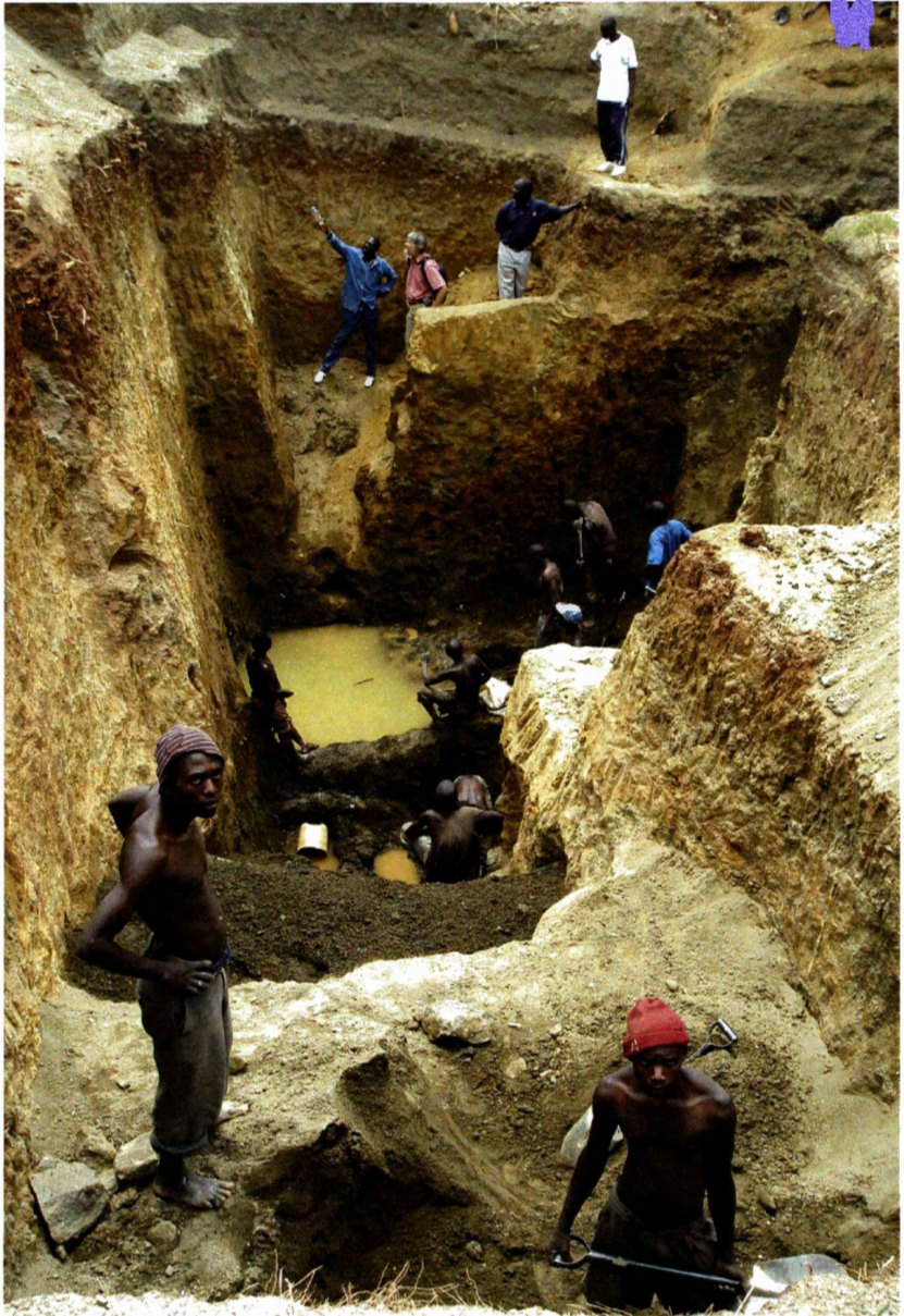
Fig. 5-4. Very deep pit with near vertical walls in a garnet mine in Lundazi area. The vertical wall in the left side of the picture may create rock fall causing serious injuries to the miners
