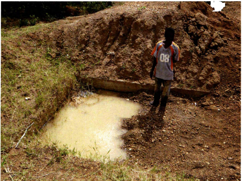
Fig. 3-6. Concrete lined basin for washing alluvial material containing spessartine. The finegrained material deposited in the basin is prevented from being washed into the drainage system
