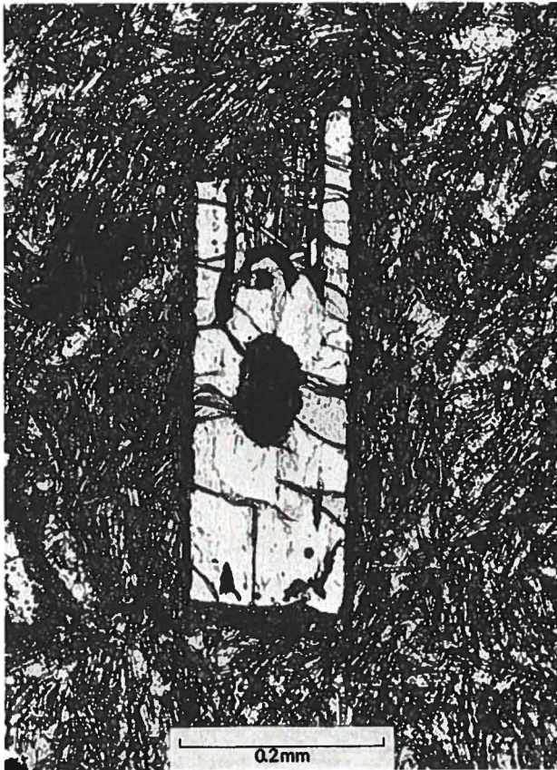
Fig. 332. Orthopyroxene phenocryst showing skeletal growth in marginal zone. From native iron bearing intermediate rock quenched when flowing into water. Asuk, Disko.
