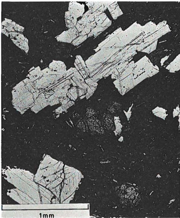
Fig. 334. Phenocrysts of plagioclase, olivine and augite in a fine-grained groundmass. Feldspar-phyric basalt from subaqueous lava tongue. Godhavn, south Disko.
