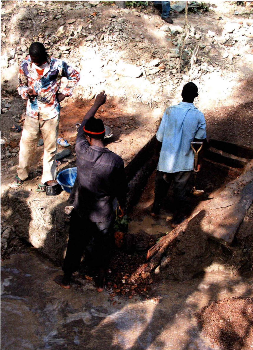
Fig. 6-1-A. A very primitive sluice where buckets of water are thrown on the upper part of the sluice. The result is that many of the heavy mineral grains (gold or tantalite) will be washed out of the sluice and get lost at Tongakura, Kogi State.
