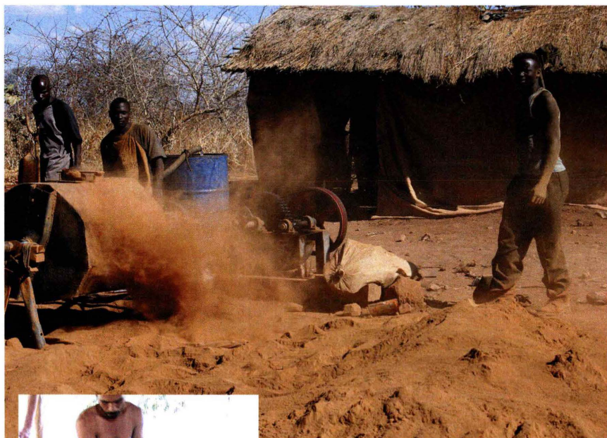
Fig. 7-1a. Dry grinding of quartz-gold ore in a ball mill produces large amounts of dust.
