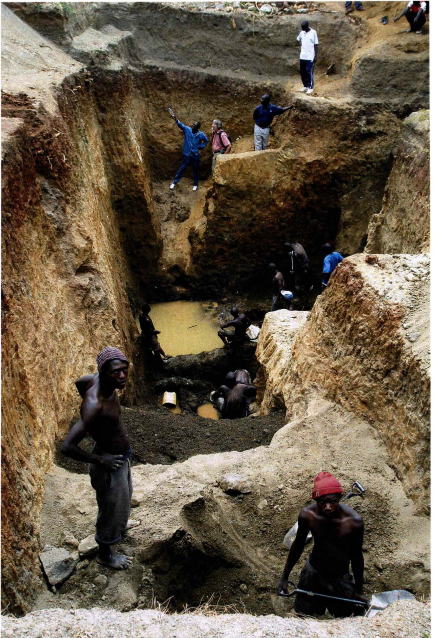
Fig. 7-10. Very deep pit with near vertical walls with a high risk of accidents caused by falling stones.
