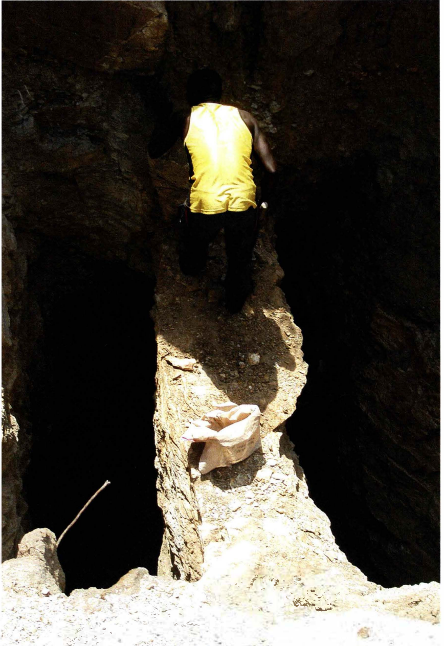
Fig. 8-2. This is a situation where all safety measures have been violated: Steep pit sides, a bridge which can collapse and stones that may fall from above. Nahuta, Gombe State.
