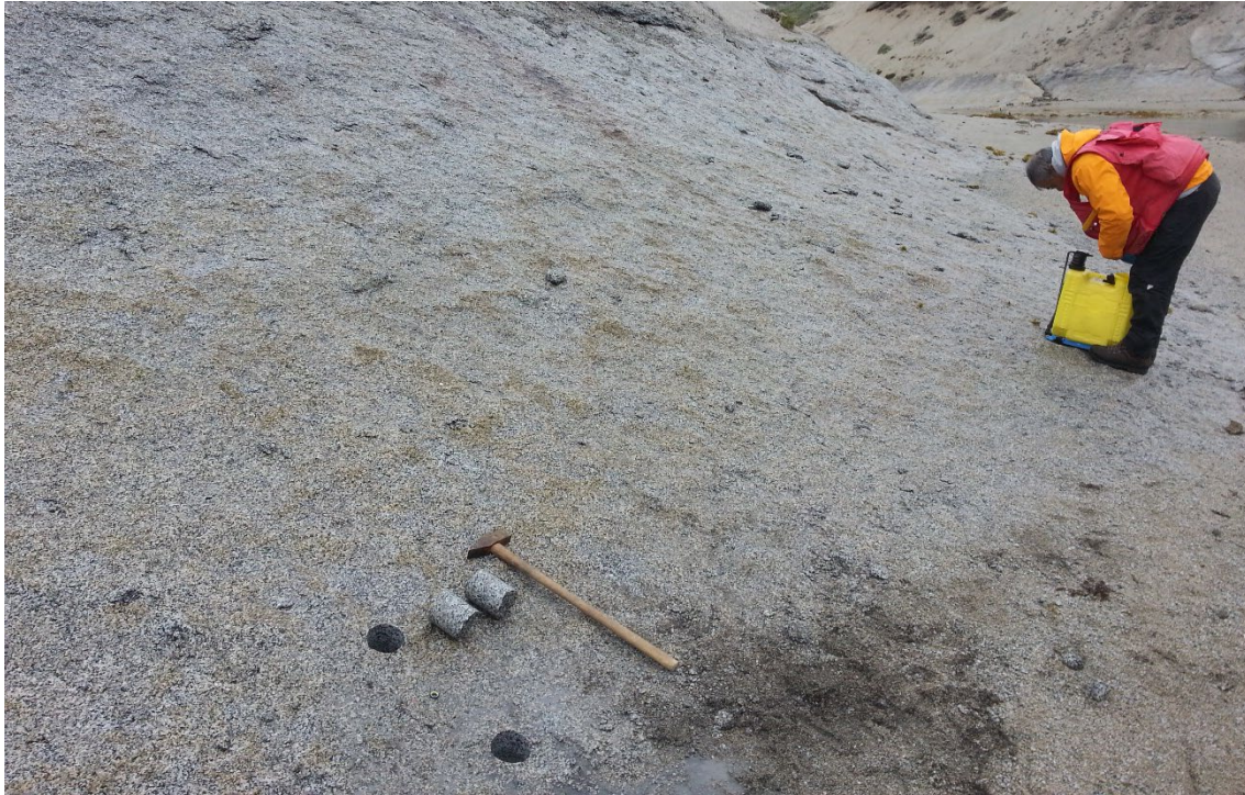
Figure 44 Syenite in the center of the Hviddal Composite Dyke (sample no. 521520) Locality 49. Very few fractures, but substantial weathering.
