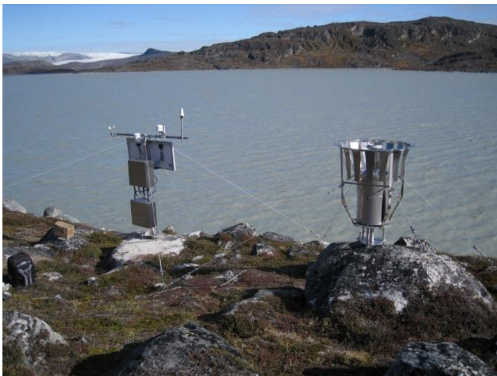
Figure 7. Hydrometric station monitoring catchment 07.d.I. Stations measures the water depth as well as selected climatic parameters (air temperature, wind speed and precipitation). The station is powered by solar panels and batteries. Data are stored in a data logger on site and transferred on a daily basis to Asiaqs office via an iridium satellite modem. Photo: Asiaq.
